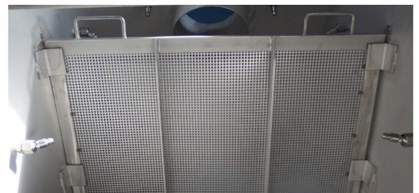
After the cleaning, the drainage of the filter is triggered by the opening of an automatic valve at the bottom of the filter. Accumulated solids and contaminants flow out the bottom drain nozzle to the sewer. A tangential water inlet nozzle helps to flush the solids remaining on the bottom surface in order to completely clean the filter.
