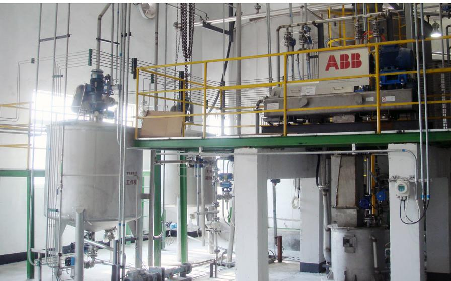
The technology of separation using centrifugation is a patent pending ABB solution which enables to recover efficiently and economically all components contained in the coating effluents in order to reuse them in the composition of fresh coating colour.
