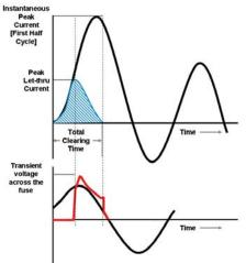
Fig. 2. Current Limiting Operation Waveforms
