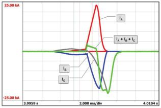
Fig. 11 – Three phase currents and  $I_0$  from Test 5.
