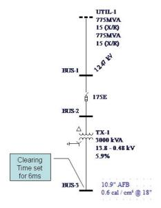
Fig. 13 - Incident Energy Calculation Example
