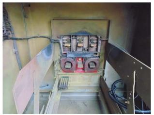
Fig. 8 – Damage to compartment from Test 9
