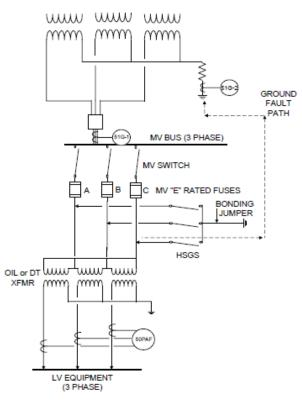
Fig. 12 - Three phase HSGS on resistive grounding system.
