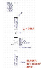
Fig. 3. Model of Incident Energy and Iarc calculations.
