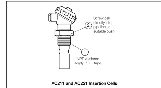
**Caution.** Overtightening may damage the cell body.
