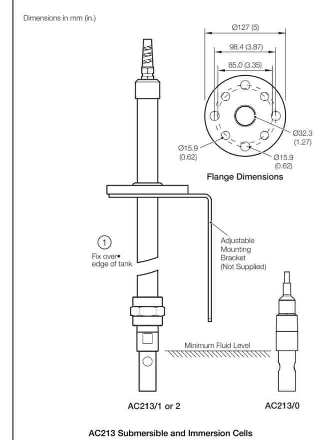
**Caution.** After cleaning and installing the conductivity cell, ensure that it remains filled with liquid and is not allowed to dry out. Ensure that the electrode bore remains fully immersed at minimum fluid levels.
