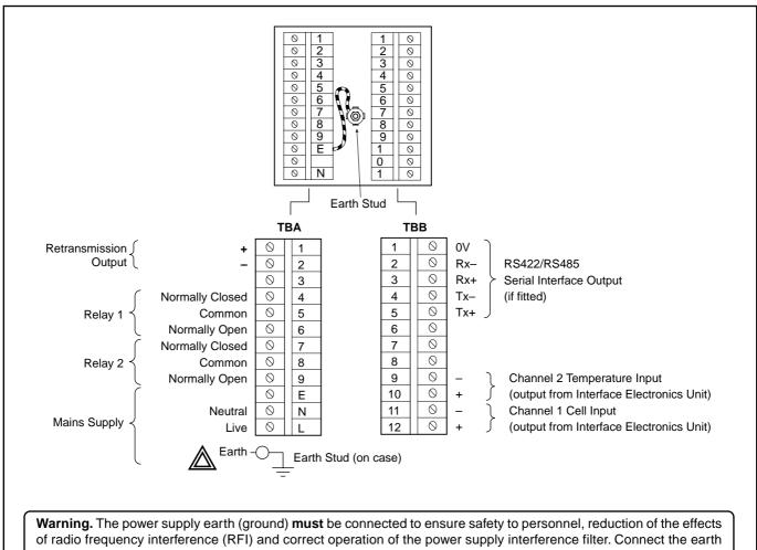
lead directly to the case earth stud and not to the 'E' terminal.
