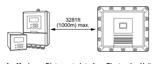
A – Maximum Distance to Interface Electronics Unit
