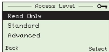
2. Press to scroll to the *Standard / Advanced* menu option and press (both passwords must be set independently). If passwords are un-set, the *Easy Setup* page is displayed:
