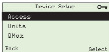
5. Press to display *Access* menu options and use the and keys to scroll to the *Standard / Advanced Password* menu (as required):
