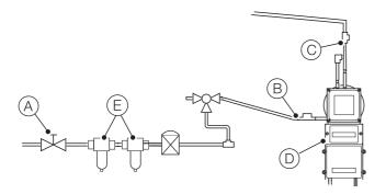
Fig. 5.2 Disconnecting instrument air and test gas supplies
