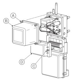
Fig. 6.1 Removing the sensor covers
