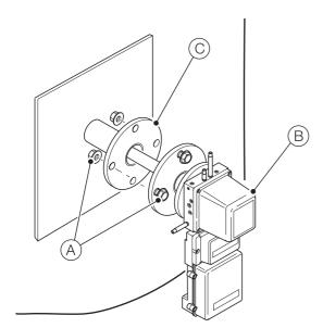
Fig. 5.4 Removing the sensor assembly from the process
