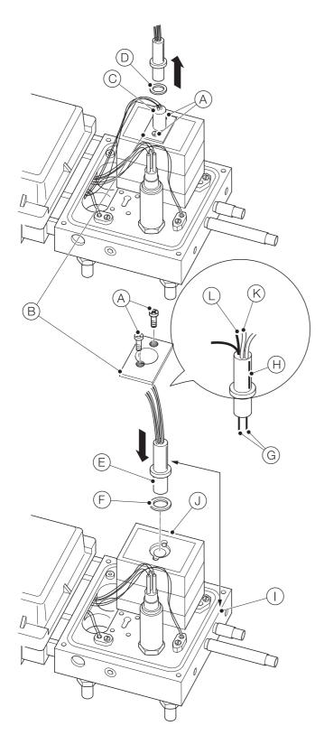
Fig. 6.3 Replacing the CO sensor
