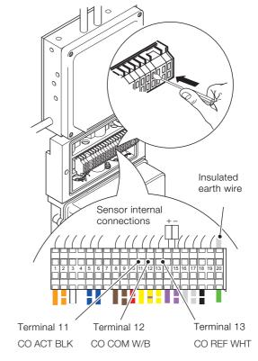
Fig. 6.2 Disconnecting the CO sensor
