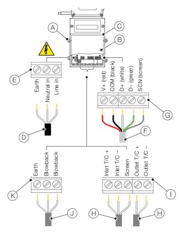
Fig. 5.3 Disconnecting sensor cables
