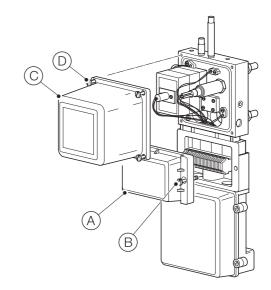
Fig. 6.5 Refitting the sensor covers
