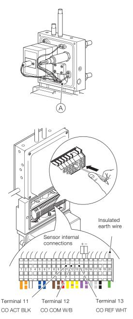
Fig. 6.4 Connecting the CO sensor
