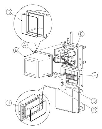
Fig. 5.1 Sensor covers replacement procedure
