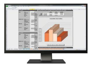
Spirit<sup>IT</sup> Flow-Xpert Excel Edition is a MS Excel spreadsheet add-in that comes with a sample MS Excel workbook containing graphical user interface. All Spirit<sup>IT</sup> Flow-Xpert calculation functions are available as MS Excel functions, which enables you to build customized applications, such as a flow computer verification tool and a meter ticket recalculation program.
