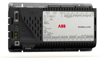
NextMove e100 features the Mint motion control language. Mint is a structured form of Basic, custom designed for stepper or servo motion control applications. It allows you to get started very quickly with simple motion control programs. In addition, Mint includes a wide range of powerful commands for complex applications.
