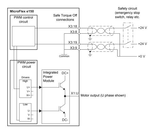
**WARNING!** The STO function does not disconnect the voltage of the main and auxiliary circuits from the drive. Therefore maintenance work on electrical parts of the drive or the motor can only be carried out after isolating the drive system from the main supply. If the drive was connected to the input power, wait for 5 minutes after disconnecting the input power.
