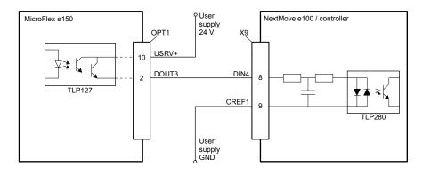
DOUT3 - typical connections to an ABB NextMove e100:
