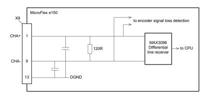
Encoder channel input circuit - channel A shown:
