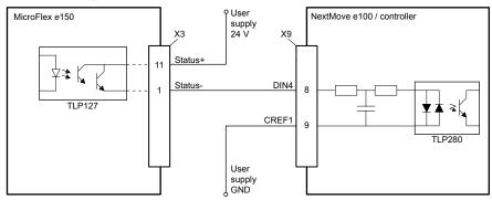
Status output - typical connections to an ABB NextMove e100:
