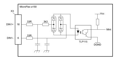
Digital input - typical connections from an ABB NextMove e100:
