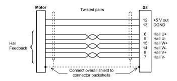
Halls-only feedback cable connections - rotary motors:
