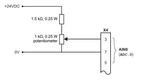
Typical input circuit to provide 0-10 V (approx.) input from a 24 V source
