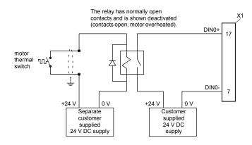
**WARNING!** The 24 V DC power supply connected to the thermal switch must be a separate supply as shown in the diagram. The thermal switch wires often carry noise that could cause erratic drive operation or damage. The thermal switch contacts must never be wired directly to a digital input. The separate 24 V DC supply used for the thermal switch can also be used for the motor brake circuit.
