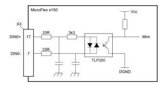
Digital input - typical connections from an ABB NextMove e100:
