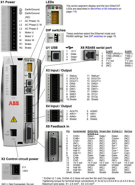
(NC) = Not Connected. Do not make a connection to this pin.
