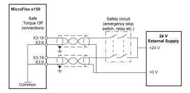
**Note:** If the contacts of the safety circuit do not open/close within 1 ms of each other, then a fault in the STO circuit or wiring is assumed and the drive will become disabled. The maximum allowed cable length between the drive and the activation switch is 30 m (98 ft).
