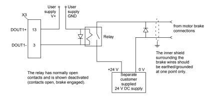
This circuit uses DOUT1 as a motor brake output. The output is configured using Mint keyword MOTORBRAKEOUTPUT; see the Mint help file for details. With this configuration, the following sequences can be used to control the brake.
