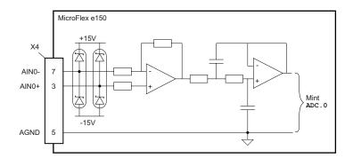
For differential inputs connect input lines to AIN+ and AIN-. Leave AGND unconnected:
