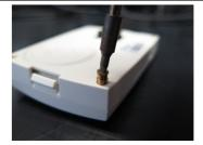
Heat the soldering iron to 350°C and heat the insert for two seconds.
