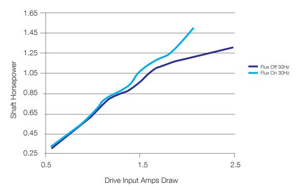
As the load was increased, the motor began to operate near the constant-torque mode. This created a large increase in efficiency, when using flux optimization. This was because the V/Hz ratio was set to the squared ratio, and the drive required additional flux to generate more torque. Flux Optimization has the ability to increase or decrease the magnetic flux in the motor to match the demand of the load.
