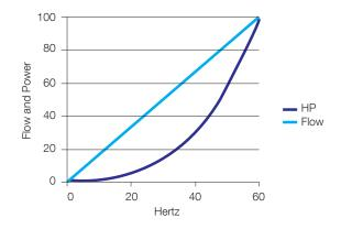
The Affinity Law states that the flow in a fan or pump application is proportional to the fan or pump speed. This results in a reduction in required motor horsepower by the cubed change in speed.
