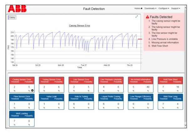
Figure 45: Fault Detection dashboard with single file analysis results
