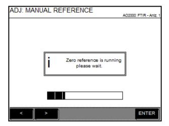
3 Once the recording of the manual reference has stopped, a message confirms if the process was completed successfully or not.
