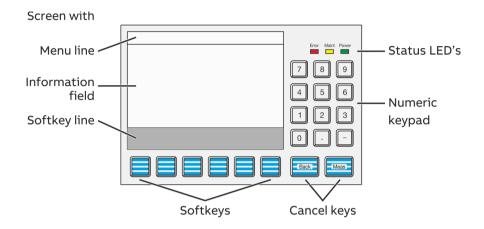
The display and operation unit consists of
