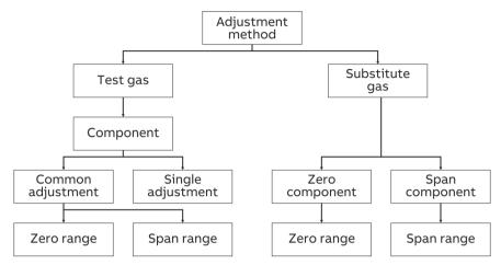
The adjustment method can be set separately for every one of the three types of controlling the adjustment (manual, automatic and externally controlled).
