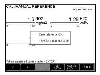
4 If the manual reference was recorded successfully, save the reference as SECURE AS LKG (Last Known Good). It is then activated in the FTIR.
