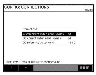
Only the enabled and configured corrections are shown in the menu. The image shows maximum configuration.
