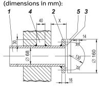
Installation of the wall tube in brickwork with metal sheeting (dimensions in mm):
