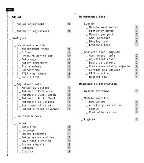
For reasons of clarity, only the suitable parameters and functions are presented; the menu links onward at most menu items, e.g. to the selection of the various measured components or to the selection and settings of values.
