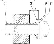
Installation of the wall tube in an insulated sheet-metal channel (dimensions in mm):
