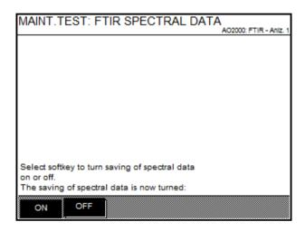
The appearance of the softkeys indicates the current status of the function. The image shows that the saving of FTIR spectral data is activated.
