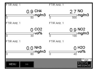
Each display "page" shows the measured values of six measuring components.
