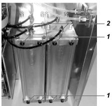
Only the two front filter cartridges must be replaced.
