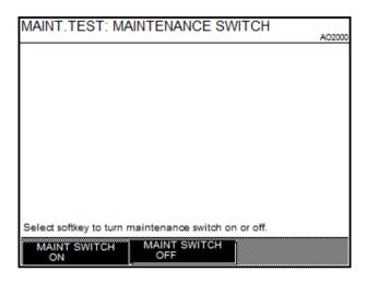
The appearance of the softkeys indicates the current status of the maintenance switch. The maintenance switch displayed in the figure above is switched on.
