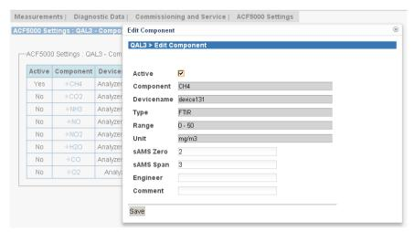
Measuring components that must be checked during the AAC can be activated and configured in the Edit Components submenu.
