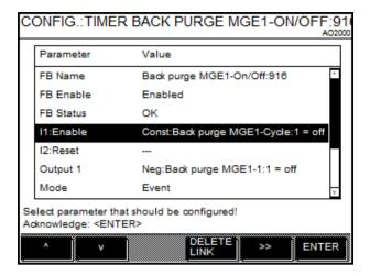
4 Activate on the selected Constant function block the back purging:
