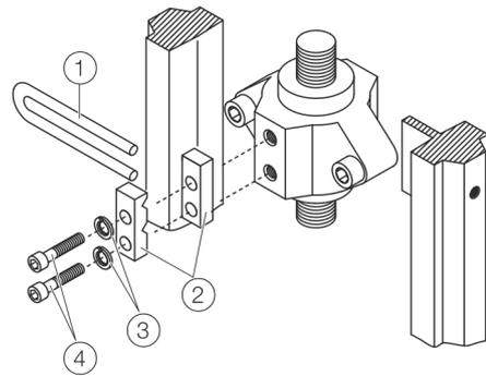
Figure 7: Attaching a follower guide to the actuator
