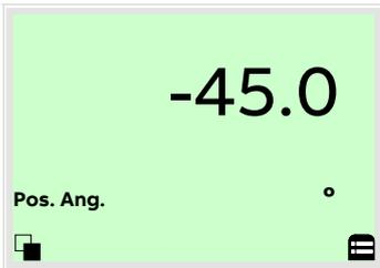
Check the end positions. The angle of rotation is displayed in degrees.
