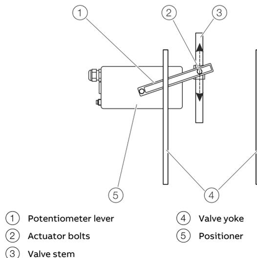
Figure 13: Actuator bolts on the valve (rear view)
