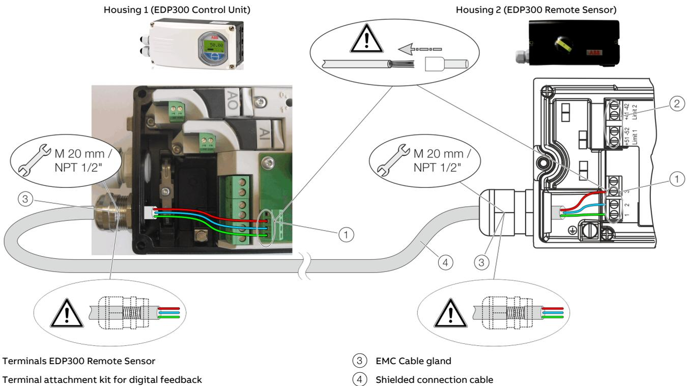
Figure 23: Connection EDP300 Control Unit with EDP300 Remote Sensor (example)
