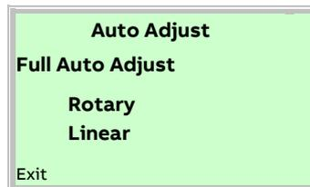
4. Use ▲ or ▼ to select 'Actuator type'. Select 'Rotary' for rotary actuators. Select 'Linear' for linear actuators.
