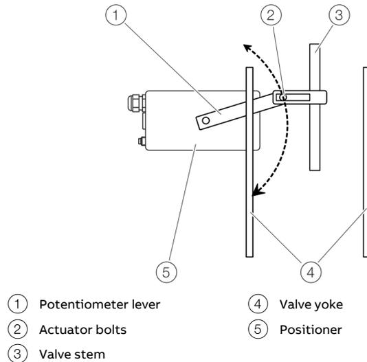
Figure 12: Actuator bolts on the lever (rear view)
