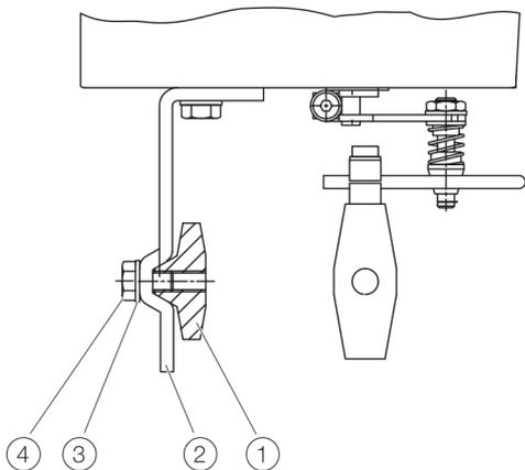
Figure 9: Mounting on a cast iron yoke
