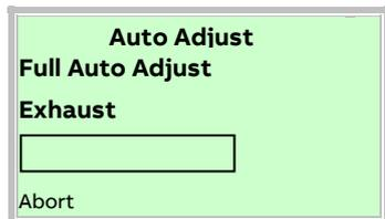
The progress of the Auto Adjust function is shown in a bar graph. The function can be terminated with 'Abort' if necessary. Once Auto Adjust has been completed successfully, 'Auto Adjust Complete' is displayed. The device then switches to the process display automatically.
