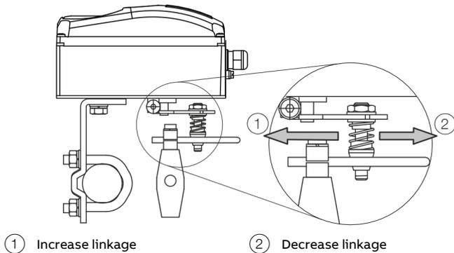
Figure 11: Positioner linkage
