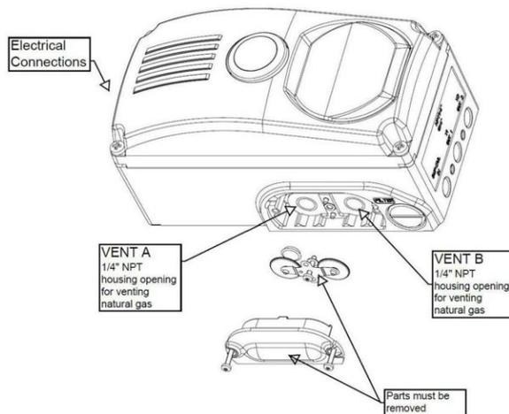
9. Vent tubing connection requirement, shown as VENT A & VENT B (above), is 1/4" NPT. The tubing size for Vent A & Vent B should match the supply tubing size.
