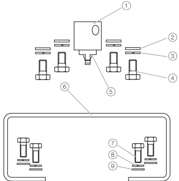
Figure 16: Components of attachment kit
