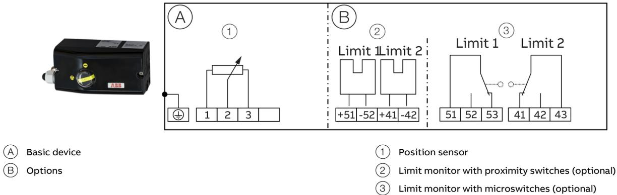
Figure 21: EDP300 Remote Sensor Electrical Connection
