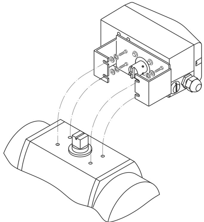
Figure 19: Screwing the positioner onto the actuator
