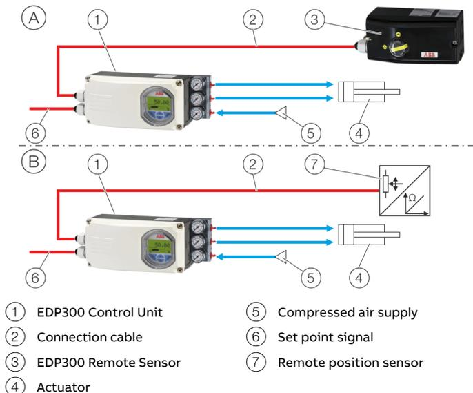
Figure 3: EDP300 with external position sensors
