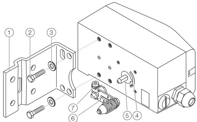
Figure 8: Mounting lever and bracket on the positioner
