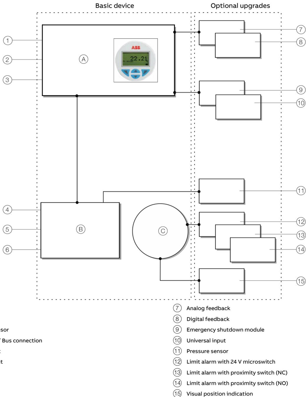
Figure 1: Schematic diagram of the positioner
