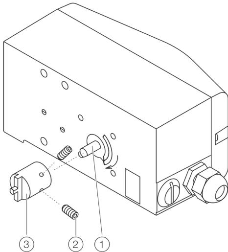
Figure 17: Mounting the adapter on the positioner
