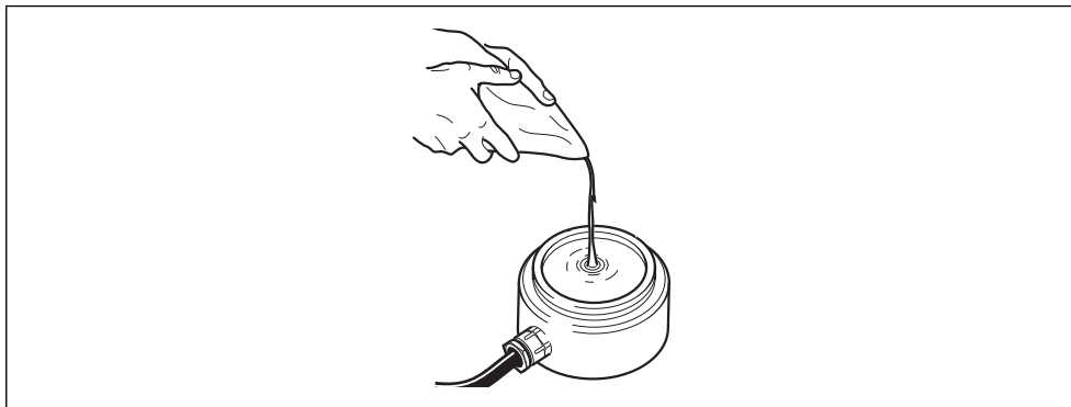
Fig. 4.2 Potting the Terminal Box – WaterMaster FET1 Transmitter
