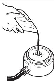
Fig. 3.10 Potting the Sensor Terminal Box
