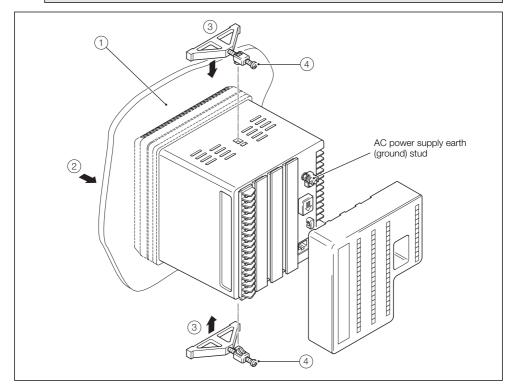
Fig. 4.4 Installing the recorder
