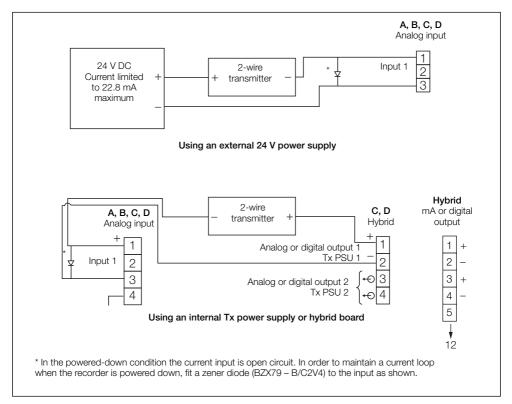
Fig. 4.8 2-lead temperature transmitter connections
