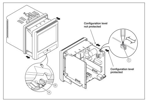
Fig. 8.3 Setting the security switch
