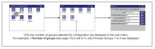
Fig. 8.9 Selecting process group configuration
