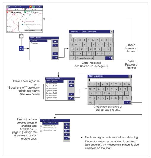
Fig. 5.13 Entering an electronic signature
