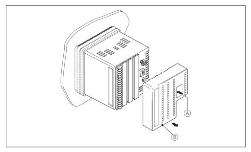
Fig. 4.5 Removing terminal cover
