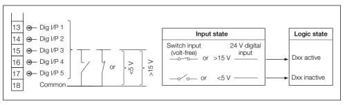
Fig. 4.9 Hybrid module digital input connections
