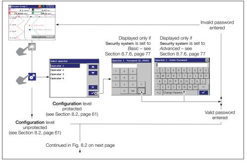
Fig. 8.1 Accessing the configuration level
