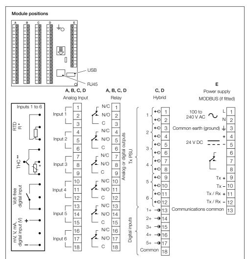
\* For 2-wire RTD connections, fit a link across the terminals where the third lead would normally be fitted.
