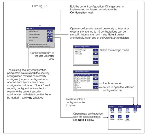
Fig. 8.2 Accessing the configuration level (continued)
