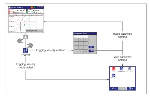
Fig. 6.1 Accessing logging - basic security
