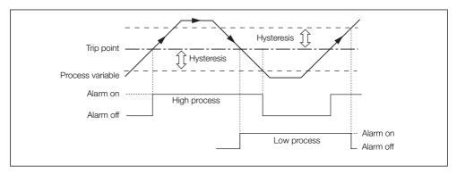
Fig. 8.11 High / Low process alarms
