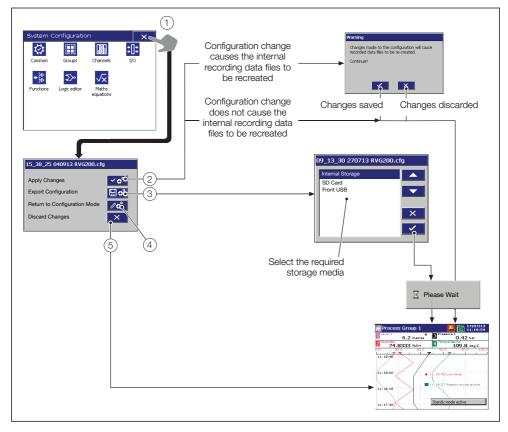
Fig. 8.7 Exiting configuration mode
