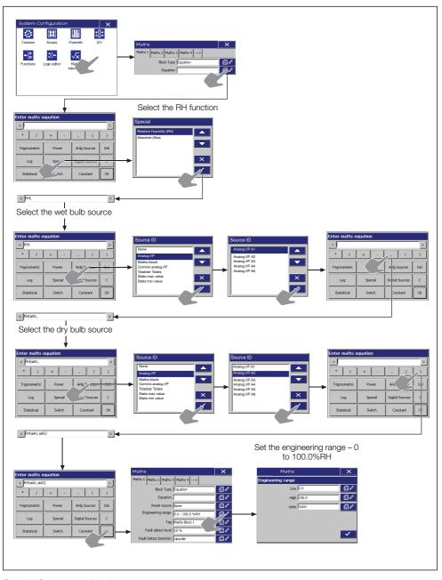
Fig. 8.22 Relative humidity calculation
