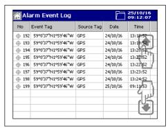
Fig. 8.18 Alarm / event log with GPS coordinate entries
