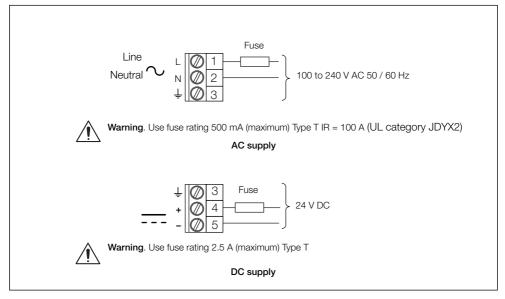
Fig. 4.7 Power supply connections
