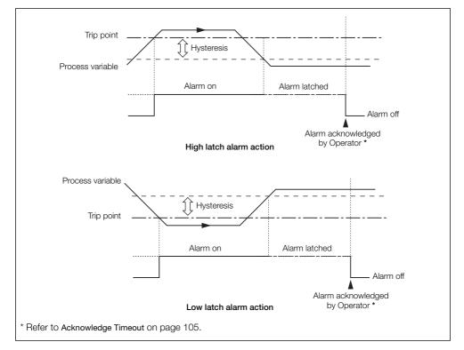
Fig. 8.12 High / Low latch alarms
