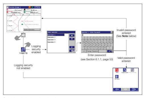
Fig. 6.2 Accessing logging - advanced security
