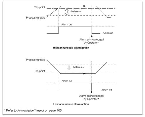
Fig. 8.13 High / Low annunciate alarms
