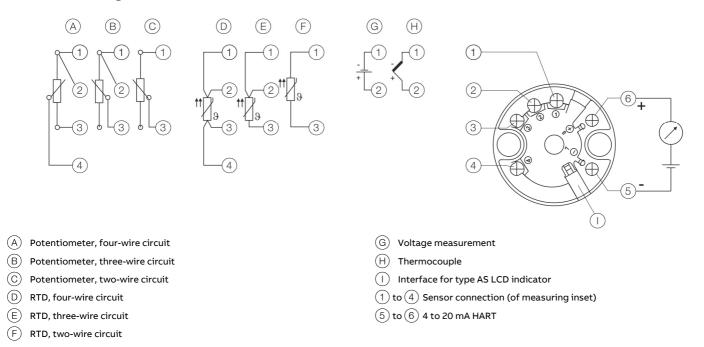
Figure 13: TTH200 connections
