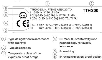
Figure 8: Additional plate for explosion-protected apparatus (example)
