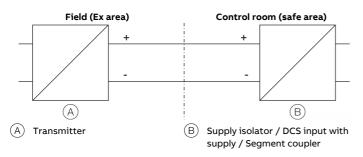
Figure 1: Intrinsic safety installation check
