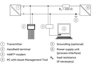
Figure 16: Example for HART connection
