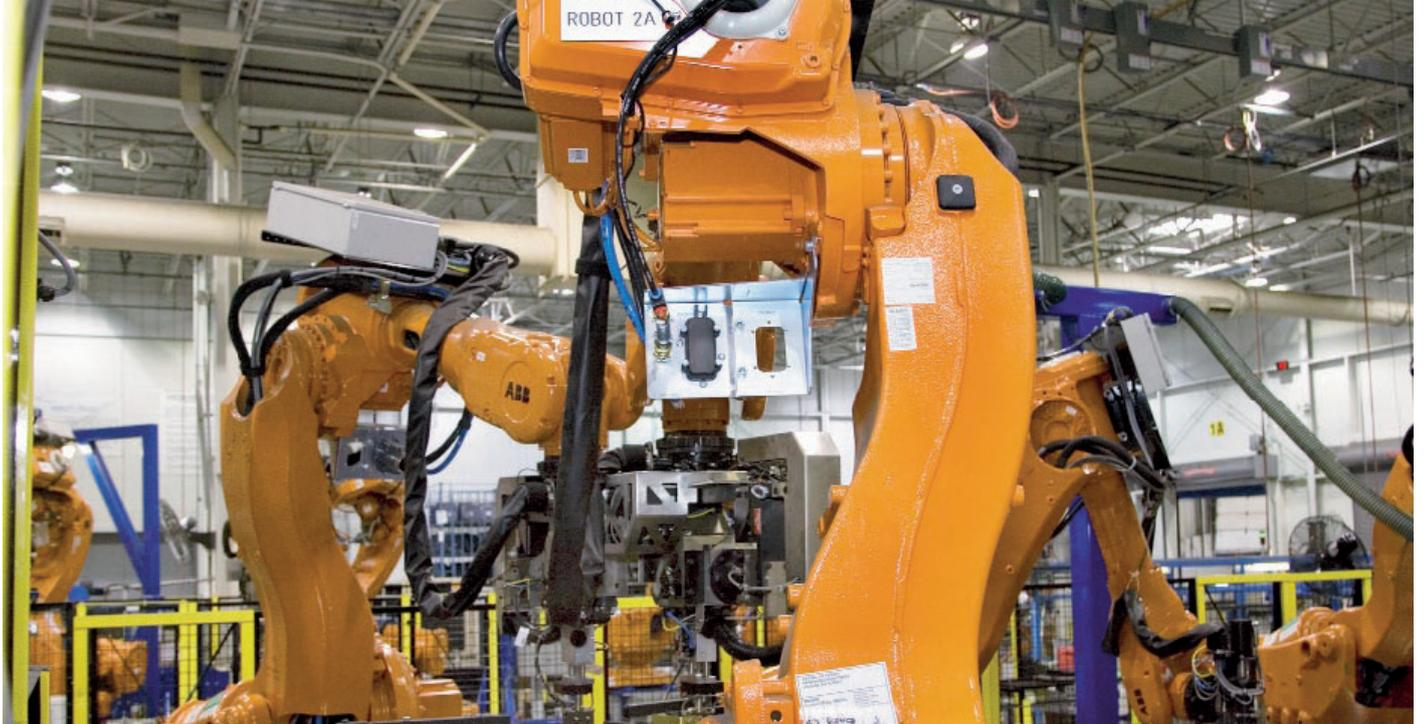
Using robots for the cutting and machine handling of plastic fuel tanks for Big Three automakers in the U.S. has given TI Automotive new speed and flexibility.
