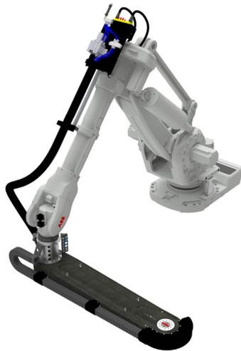
The benefits of traditional robot automation are enhanced by the addition of a rotational 7th axis. Thanks to the 7th axis, the robot keeps the orientation of the part when transferring it from the press to the next. This entails lower inside-press time occupation and better overlapping between loading and unloading robots.
