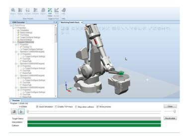
be customized to match different machine setups. It fully supports 5-axis APT/ISO standard G-Code which is also extendable via templates. Multiple strategies can be applied when calculating the target configuration of the imported CNC code. Users can also verify and modify the robot path offline before exporting to RAPID. The user interface design follows Computer Aided Manufacturing (CAM) style, is able to reflect the CAM engineer's background, and is easy to use with minimum requirements.
