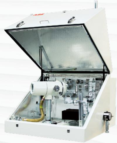
The Liquid Injection System is fully compliant with GPA 2177, as the liquid sample valve is outside the heated zone (GC). The Liquid Injection System comes as a fully integrated package, including the Liquid Inject panel, pilot valves and controller, in an environmental enclosure. Designed for NGL's with dew point below 100°C/212°F.
