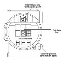
HART hand-held communicator may be connected at any wiring termination point in the loop, providing the minimum resistance is 250 ohm. If this is less than 250 ohm, additional resistance should be added to allow communications.
