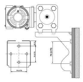
• 621SS transmitter with welded flanges on flat type (for box) bracket for vertical or horizontal 60 mm (2in) pipe mounting
