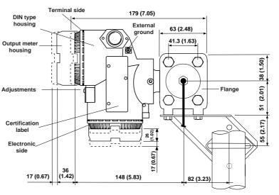
621SS transmitter with welded flanges on bracket for vertical or horizontal 60 mm (2in) pipe mounting
