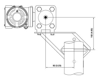
• 621SS transmitter with welded flanges on bracket for wall mounting (by four M8 screws)
