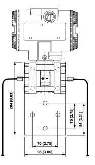
624SS transmitter on bracket for 60 mm (2in) pipe mounting (barrel housing)
