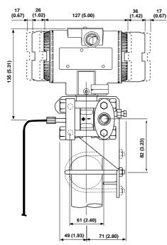
NOTE : For 621SS side with 1/2"-14 NPT threaded process flange connection, gasket groove and gaskets are in accordance with DIN 19213; removing adapter the flange provides a direct 1/4"-18 NPT thread. Bolting threads for fixing adapter or other devices (i.e. manifold etc.) on process flange is 7/16"-20 UNF.
