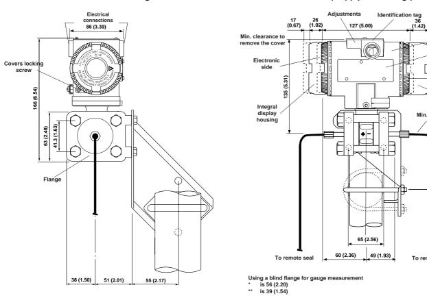
Dimensions of positive and negative side can be inverted according to high and low pressure side code selections. Selecting one side with blind flange (for gauge) or vacuum reference, consider one capillary only to remote seal
