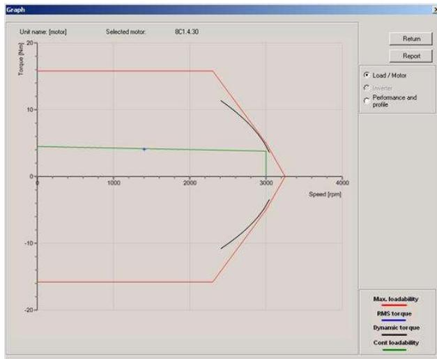
Figure 58 Motor Graph display for ServoMotor
