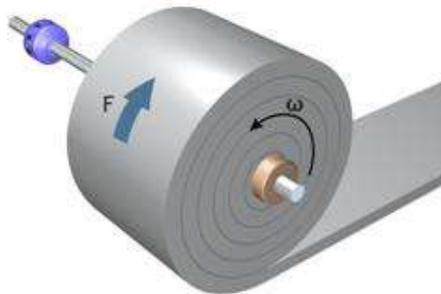
Figure 49 Unwinder mechanics.
