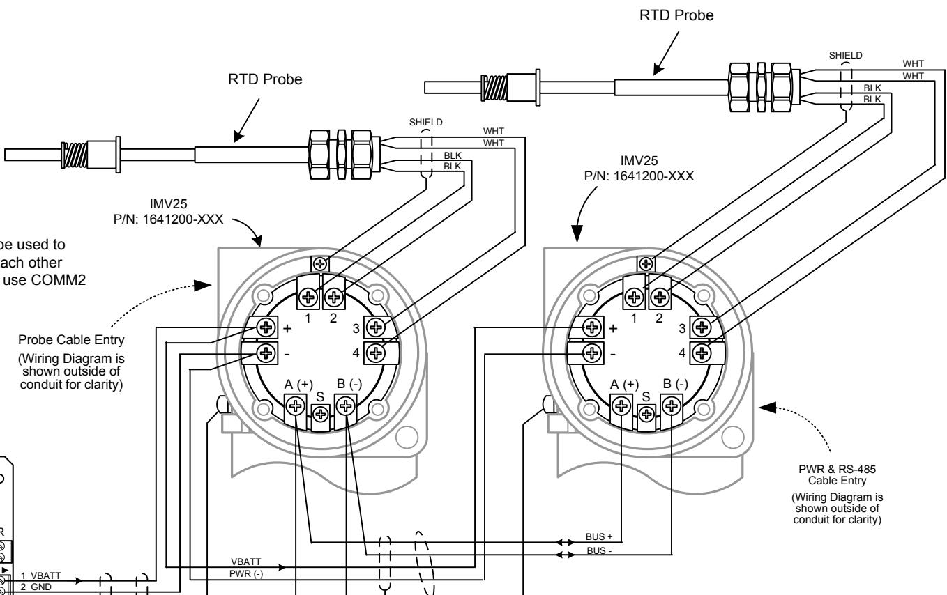
Connect the Shield GND from the RS-485 cable at the enclosure end of the cable to the Chassis GND Lug located on the bottom of the enclosure. For every other RS-485 cable to an additional device, attach Shield GND to Shield GND. DO NOT ground at any other place.
