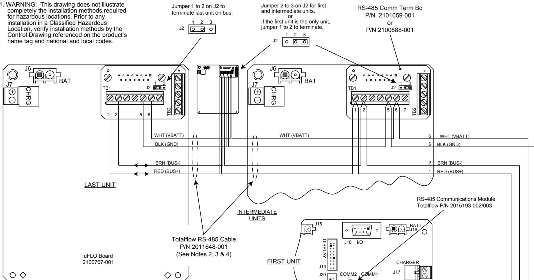
2. Maximum length of RS485 bus is 4000 Ft. @9600 baud using Totalflow cable P/N 2011648-001 or equivalent.
