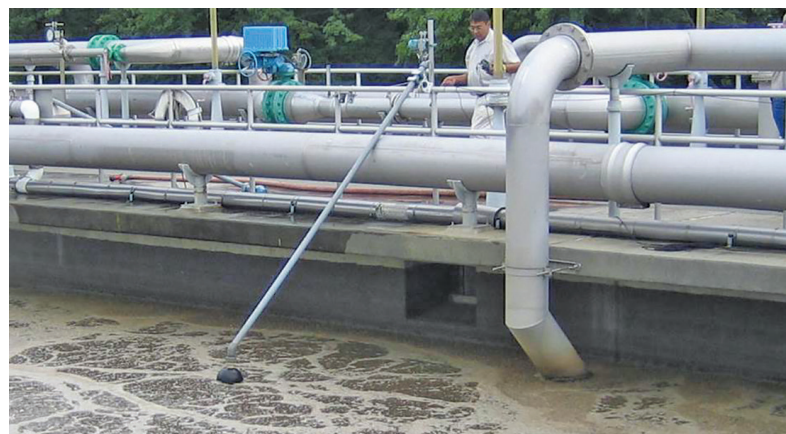
Figure 2 A floating ball-type DO sensor shown measuring in situ
