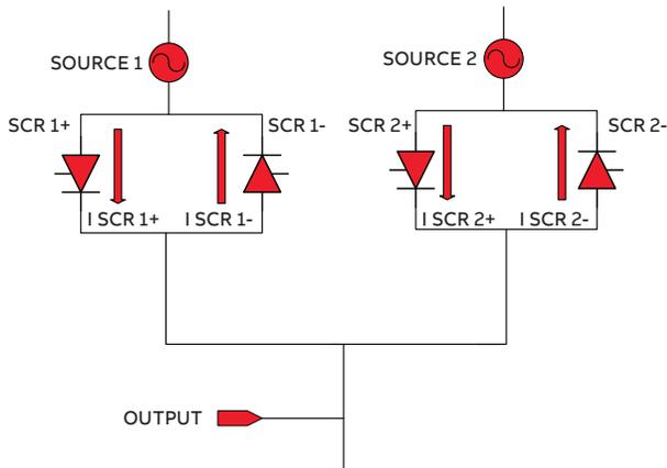
Figure 15: Static Transfer Switch and A9 algorithm
