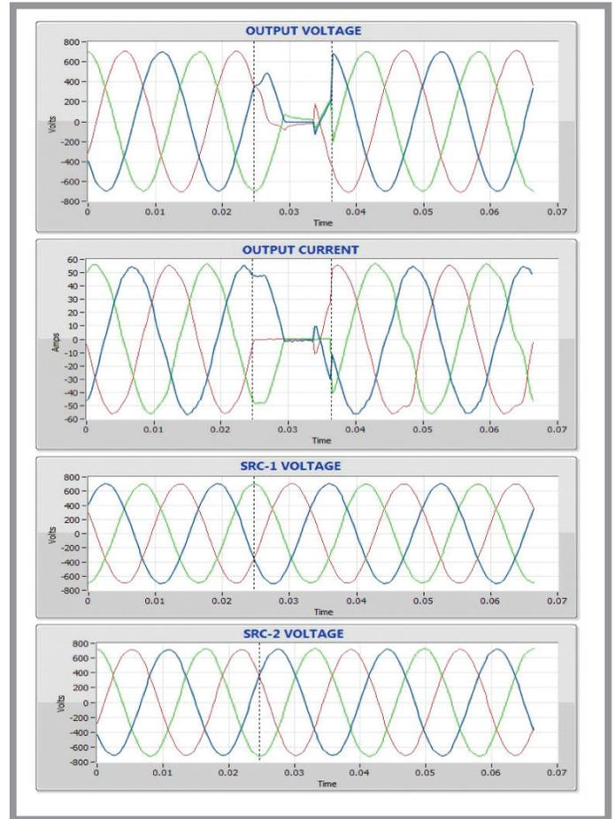
Figure 12: Phase: 180 degree, outage time: 11.50 ms
