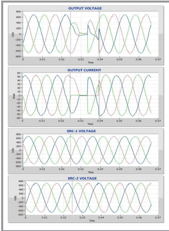
Figure 11: Phase: -60 degree, outage Time: 14.50 ms
