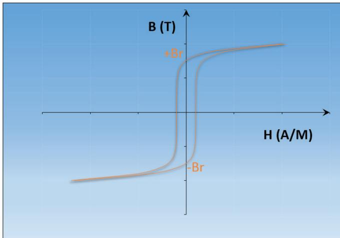
Figure 3: B-H curve of a power transformer
