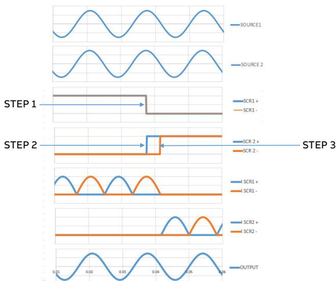
Figure 16: A seamless A9 transfer, synchronized sources
