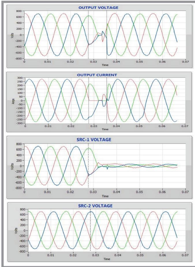
Figure 9: Phase: -120 degree, outage time: 8.00 ms
