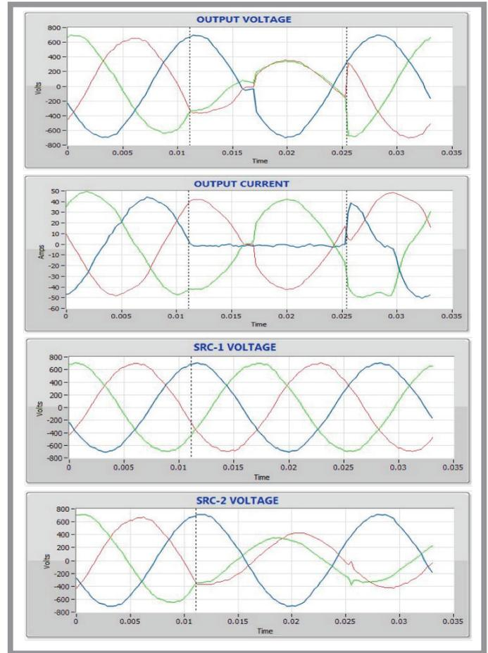
Figure 10: Phase: 0 degree, outage time: 14.50 ms
