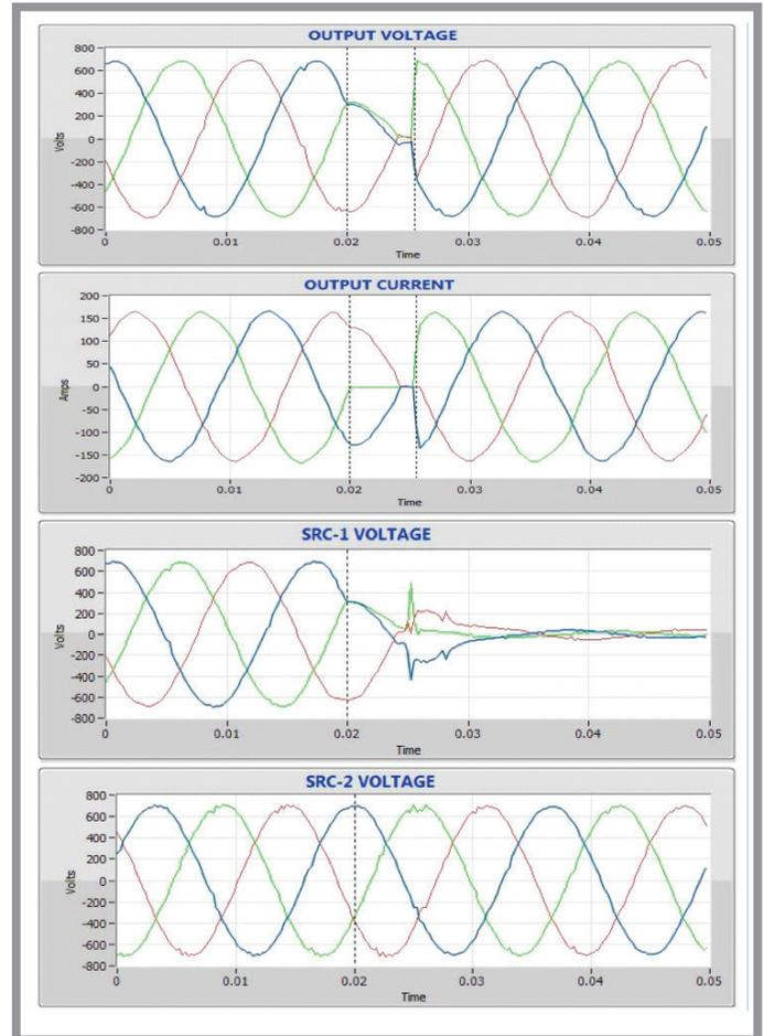
Figure 8: Phase: 60 degree, outage time: 5.50 ms
