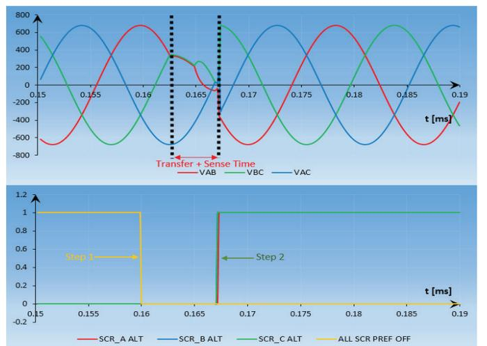
Figure 6: Steps required to do a super transfer
