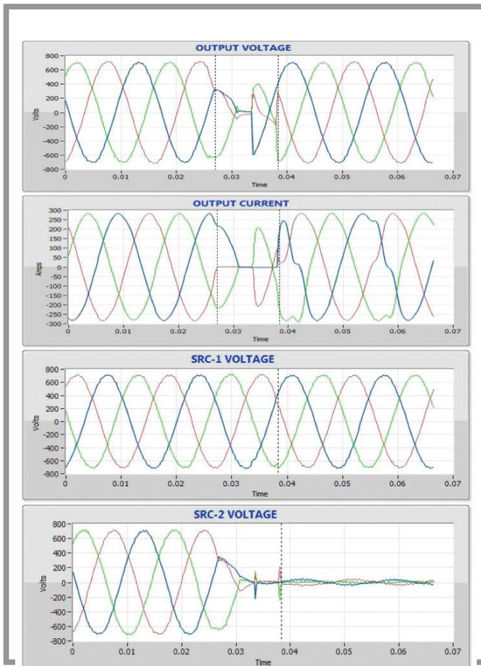
Figure 7: Phase: 120 degree, outage time: 11.50 ms
