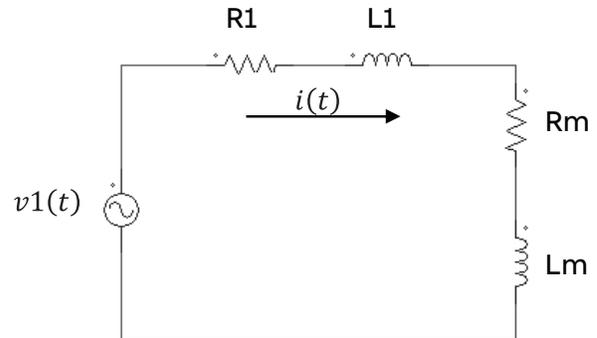
Figure 2: Equivalent Circuit of an unloaded transformer.
