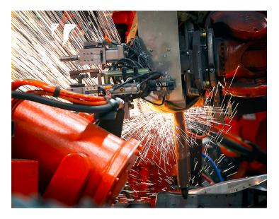
Figure 4: Diodes are stressed by regulated short circuit during weld spot.
