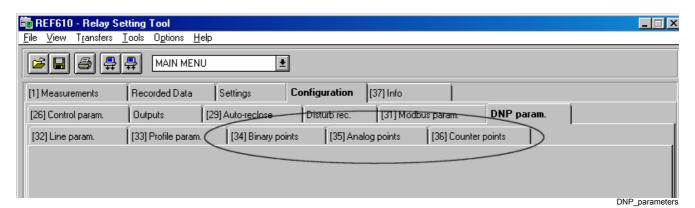
Fig. 12.1.-1 The DNP parameters of the Relay Setting Tool
