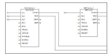
Fig. 2.4.2.4.-2 Example of a function block configuration where the nominal currents are connected to the  $I_{\rm n}$  inputs and the  $I_{\rm o}$  current is connected to the  $I_{\rm o}$  input in the function block.
