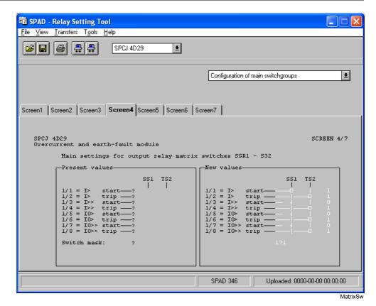
Fig. 4.4.2.3.-3 The main settings for output relay matrix switches of the module SPCJ 4D29.
