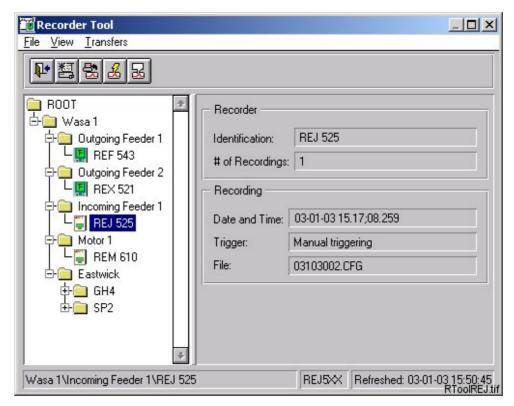
Fig. 7.3.7.-1 An example of a Recorder Tool main view with the tree structure and information concerning the internal disturbance recorder of REJ 5xx (or REx 61x) relay modules.
