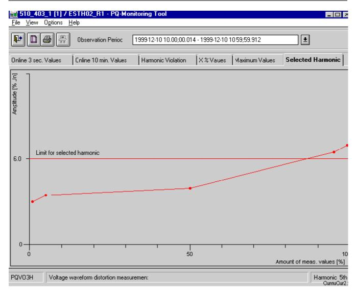
Fig. 10.3.4.-3 A cumulative curve of selected harmonic during an Observation Period (Requirements not fulfilled)
