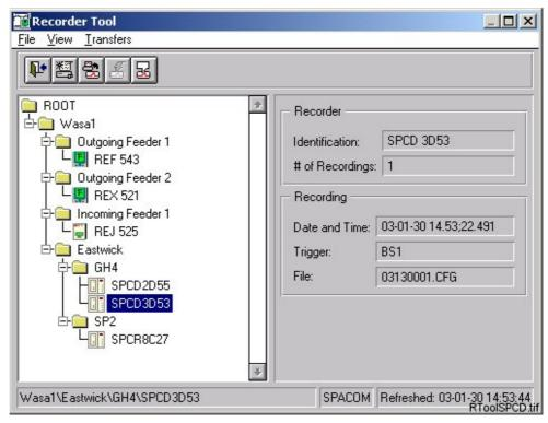
Fig. 7.3.6.-1 An example of a Recorder Tool main view with the tree structure and information concerning the SPCD 3D53 relay module.
