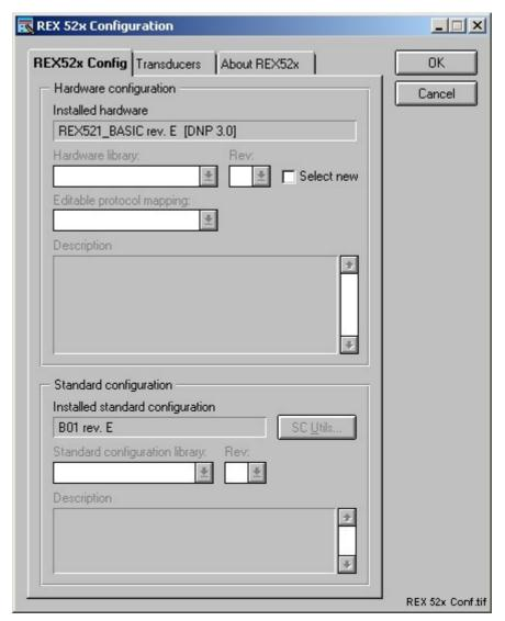
Fig. 2.4.2.1.-1 REX 52x Config page is divided into two sections: Hardware configuration and Standard configuration.
