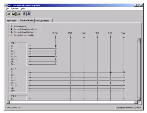
Fig. 6.4.1.2.-2 An Output Matrix showing "Connected and latched" connections
