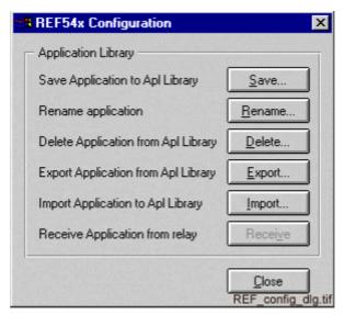
Fig. 2.4.1.4.-1 Application library utilities. The Receive function is not available in LIB 500 environment.
