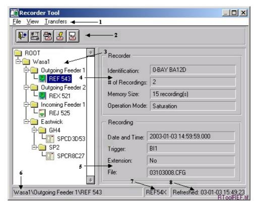
Fig. 7.3.2.-1 An example of a Recorder Tool main view with the tree structure and information concerning the MEDREC16 disturbance recorder configured for REF 54X relay.
