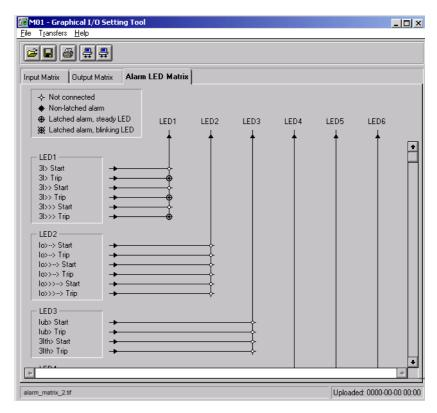
Fig. 6.4.1.3.-2 An Alarm LED Matrix showing "Latched alarm steady LED" in switchgroup LED1.
