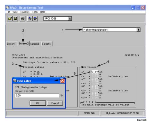
Fig. 4.4.2.3.-1 Setting Tool view
