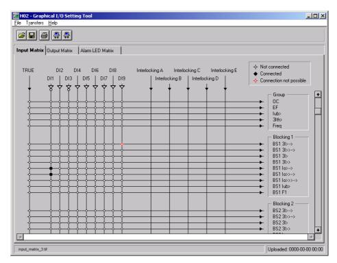
Fig. 6.4.1.-3 An Input Matrix in which a connection of DI9 input to Blocking I switchgroup is impossible.
