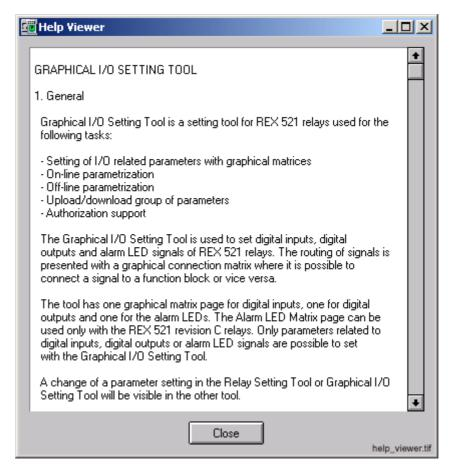
Fig. 6.4.4.1.-1 Graphical I/O Setting Tool Help Viewer dialog
