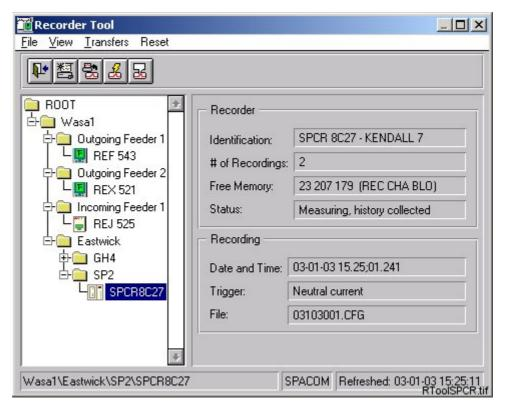
Fig. 7.3.5.-1 An example of a Recorder Tool main view with the tree structure and information concerning the SPCR 8C27 disturbance recorder configured for SPACOM relay.
