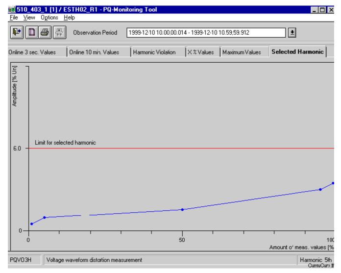
Fig. 10.3.4.-2 A cumulative curve of selected harmonic during an Observation Period (Requirements fulfilled)
