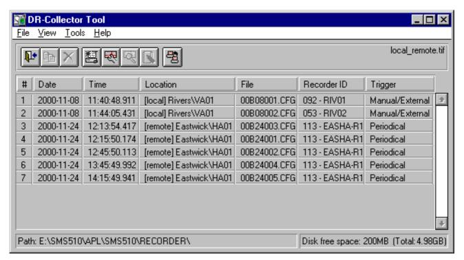
Fig. 7.4.-1 Disturbance recording list in the DR-Collector Tool. Both remotely and locally stored recordings are displayed.
