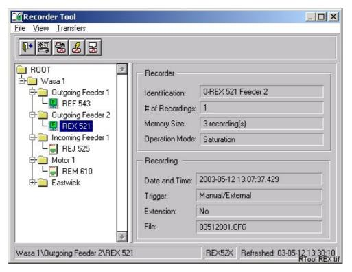
Fig. 7.3.4.-1 An example of a Recorder Tool main view with the tree structure and information concerning the internal disturbance recorder of REX 521 relay module.
