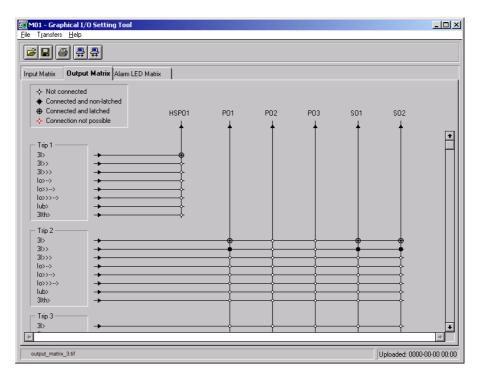
Fig. 6.4.1.2.-3 An Output Matrix showing "Connected and non-latched" and "Connected and latched" connections.
