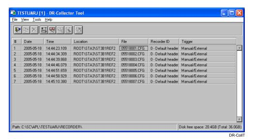
Fig. 7.2.3.-2 DR-Collector Tool presented with a list of recordings
