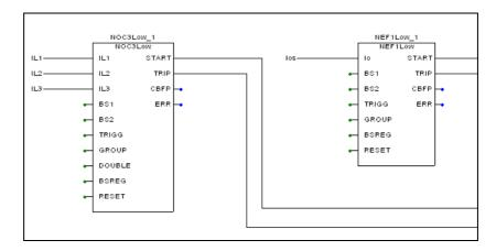
Fig. 2.4.1.6.-2 Example of function block configuration where the  $I_{\rm n}$  inputs are connected to  $I_{\rm n}$  inputs on the function block and the  $I_{\rm o}$  inputs are connected to  $I_{\rm o}$  function block inputs.
