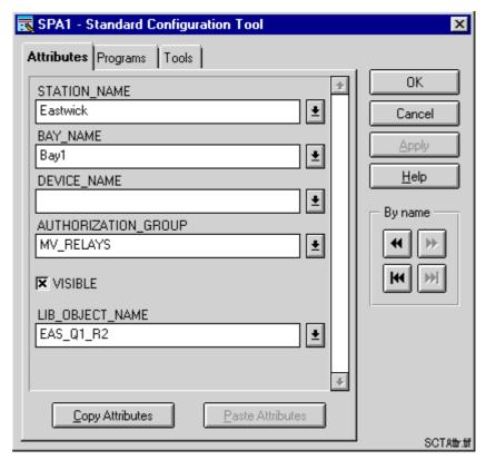
Fig. 3.3.1.3.-1 Standard Configuration Tool dialog with focus on Attributes page
