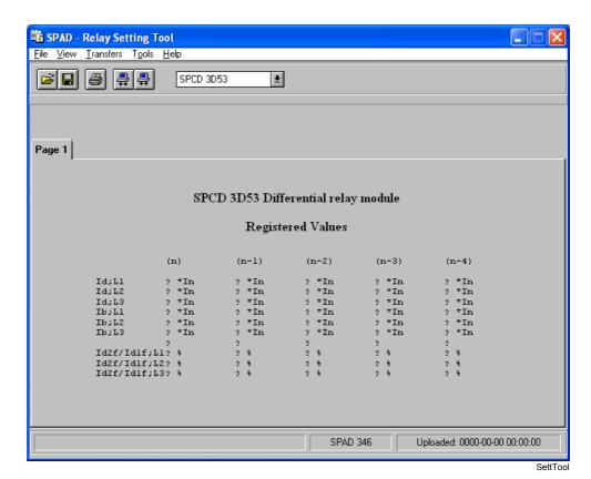
Fig. 4.4.2.2.-1 Registers View for SPCD 3D53
