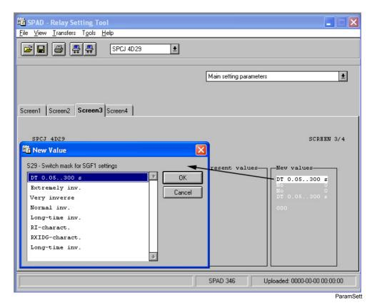
Fig. 4.4.2.3.-2 The dialog presenting possible alternatives for the new value in the Setting Tool view for main switches of the relay module SPCJ 4D29.
