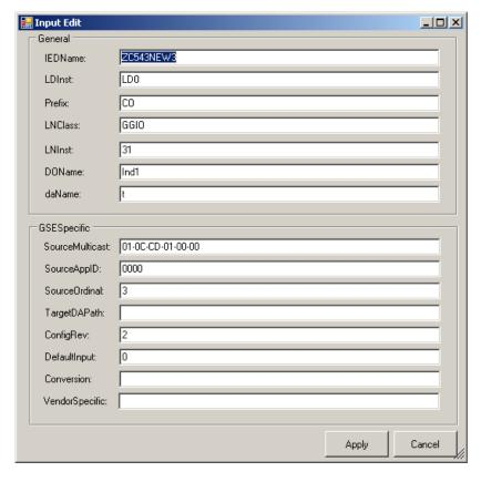
Fig. 6.11.2.1.-3 Dialog box for adding information to GOOSE Input Editor
