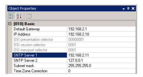
Fig. 6.7.-1 General communication parameters
