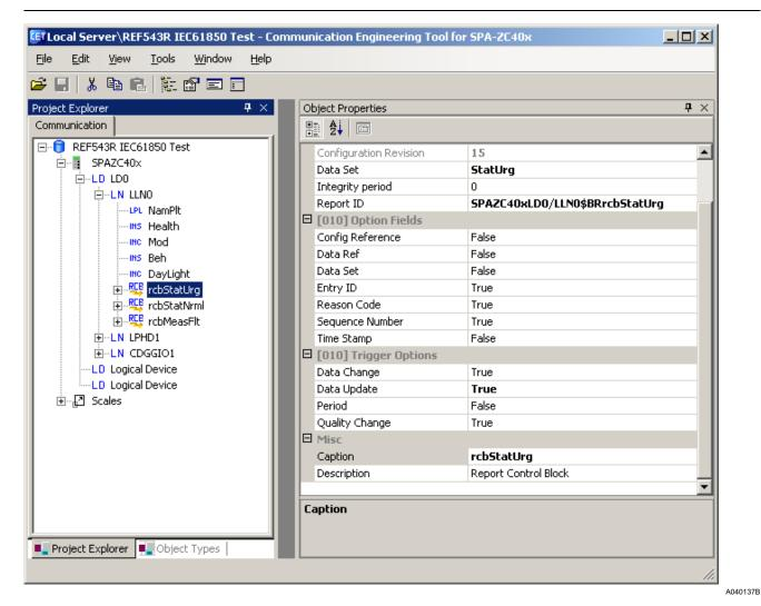
Fig. 6.4.-1 Example view of the SPA-ZC 40x Communication Engineering Tool
