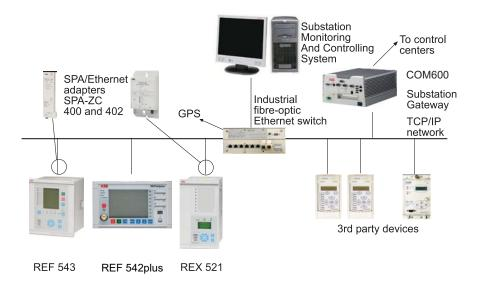
Fig. 4.-1 Conceptual picture of a typical system setup
