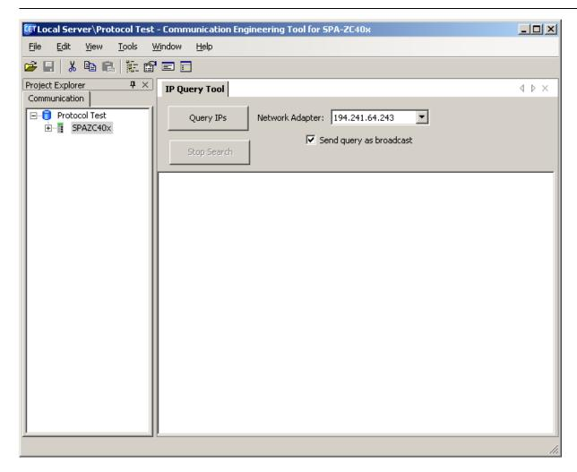
Fig. 9.3.-2 Selecting Network adapter
