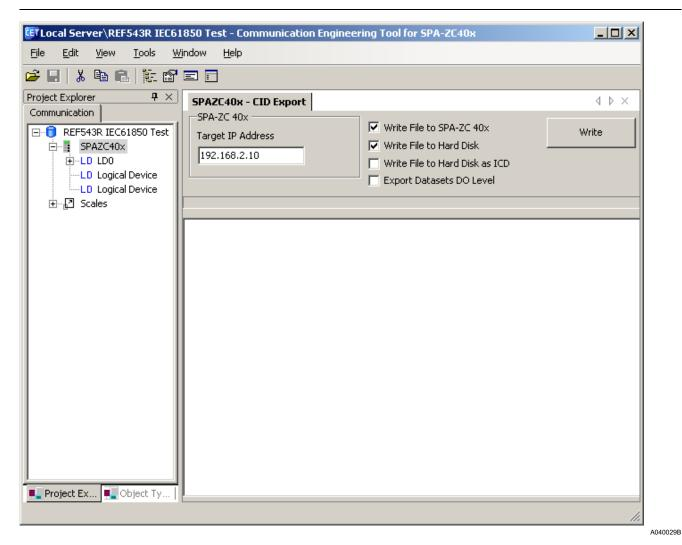
Fig. 6.8.-1 Downloading the device's configuration
