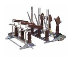
NALFWind is a 36 kV air-insulated switch-fuse combination for protection of distribution transformers in renewable installations. It is equipped with fast-acting ABB CEF-S current limiting fuses that provide protection on both MV and LV sides for transformers up to 3,000 kVA.
