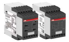
The CM-IWx series offers an innovative insulation monitoring device. In combination with a new measurement principle, networks up to 1000 V DC or 690 V AC (15-400 Hz monitor range) can be measured.
