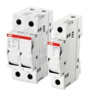
The E 90 PV series of fuse disconnectors has been designed for up to 1000 V DC applications in DC-20B category. The E 90 PV series is specifically focused on overcurrents protection of photovoltaic systems. It provides a reliable, compact and effective solution due to its  $10.3 \times 38 \, \text{mm}$  gPV cylindrical fuses.
