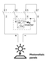
The S200 M UC Z range of miniature circuit-breakers features permanent magnets on the internal arcing chutes able to extinguish an electric arc of up to 440 V DC acc. to IEC 60947-2 with Icu = 10 kA. However, use of these components establishes circuit-breaker polarity, thus they must be powered in a certain direction. A diagram showing how the string and inverter must be connected is given alongside.
