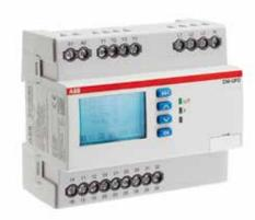
The CM-UFD.Mxx is a multifunctional grid feeding monitoring relay. It trips the section switch which is connected between the distributed generation and the public grid in order to disconnect the distributed generation in case of problems (e.g. unstable grid), faults or maintenance on the grid. Totally configurable, it offers the flexibility needed for integrate medium and small networks into main systems.
