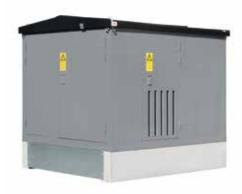
Type-tested, arc-tested assembly comprising an enclosure containing medium-voltage switchgear, distribution transformers, low-voltage switchboards, connections and auxiliary equipment to supply LV energy from MV systems.
