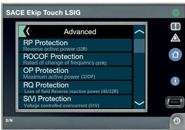
These integrated generator protective functions can be used to replace costly and bulky external generator protective relays and wiring thus saving time and money for the equipment builder without sacrificing functionality.
