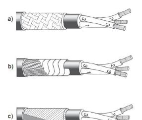
Figure 60: shield in conductive mesh a), with wound conductor b), wrapped in a helical fashion c)
