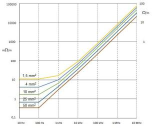
Figure 53: impedance in relation to frequency in certain cables
