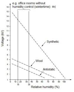
Figure 14: typical electrostatic discharge levels
