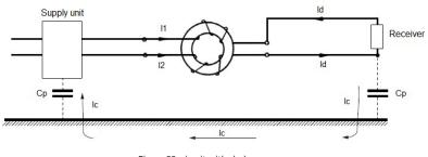
Figure 29: circuit with choke
