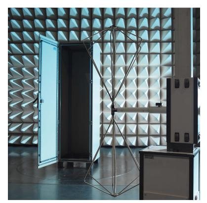
Figure 78: the ABB semi-anechoic chamber at Dalmine
