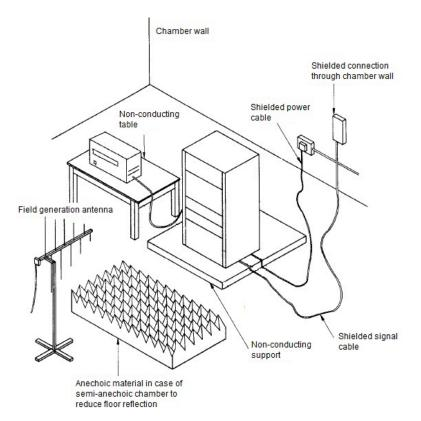
In view of the amplitude of the signal, these tests must be conducted in shielded environments so as not to interfere with the radiocommunications. The laboratory measuring instruments must also be shieldeed. The tests are typically performed in anechoic or semi-anechoic chambers that are large enough to contain the tested apparatus.
