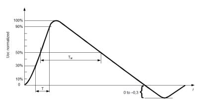
Figure 20: normalized waveform of a voltage surge
