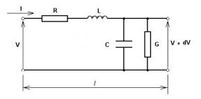
Figure 52: diagram of a conductor
