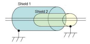
Figure 64: earthing of a cable with double shield
