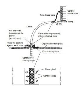
Figure 50: example of a correct connection
