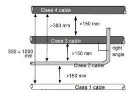
Figure 57: diagram of minimum distances between cables of different classes  $% \left( {{{\rm{cl}}_{\rm{s}}}} \right)$
