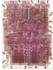
Figure 3: a) The point-contact transitor invented in 1947, b) integrated circuits, c) the first monolithic microprocessor, Intel 4004 (1971)
