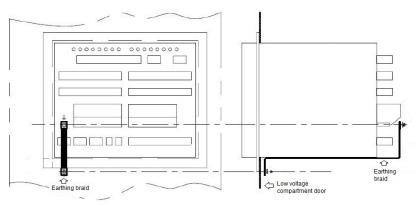
Figure 54: example of the earth connection of an IED
