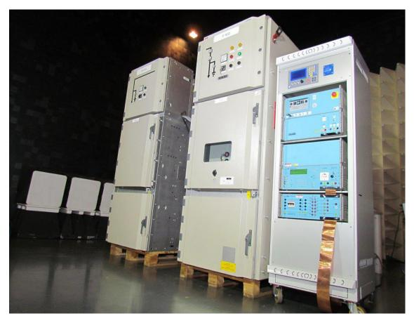
Figure 80: MV switchgear being tested in the ABB Dalmine EMC lab
