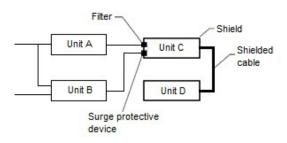
Figure 42: distributed protection system
