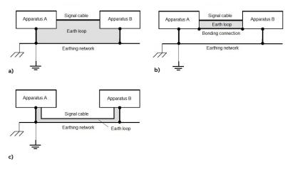
Figure 71: various ground loop configurations
