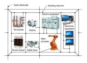
Figure 70: example of separation into zones in a building
