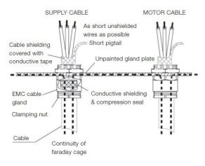
Figure 47: earthing with cable gland
