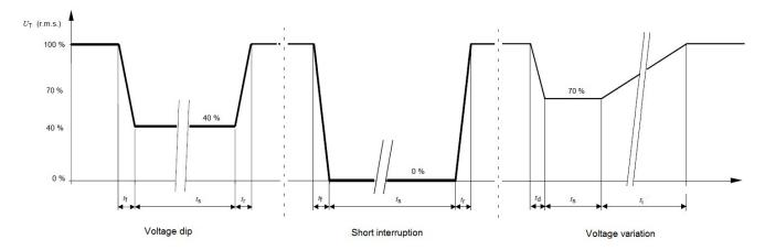
Figure 23: examples of voltage disturbance
