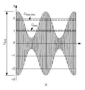
Figure 16: Waveform of severity level 1: a) non-modulated RF signal with U<sub>pp</sub> = 2.8 V and U<sub>rms</sub> = 1.0 V b) modulated RF signal with U<sub>pp</sub> = 5.1 V, U<sub>rms</sub> = 1.15 V and U<sub>max rms</sub> = 1.8 V
