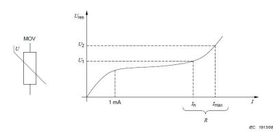
Figure 36: typical curve of a zinc oxide varistor (MOV)
