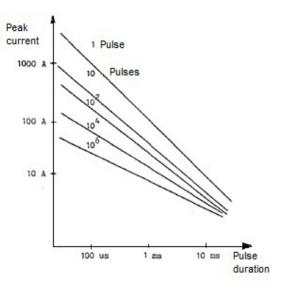
Figure 37: curves of the current peak supported by a varistor
