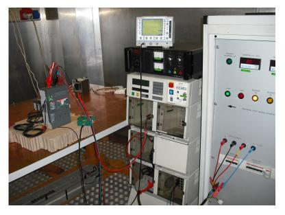
Figure 76: the shielded chamber for conducted tests
