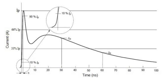
Figure 15: normalized waveform for ESD
