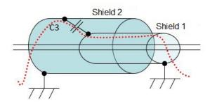
Figure 66: route taken by disturbance in a cable with double shield
