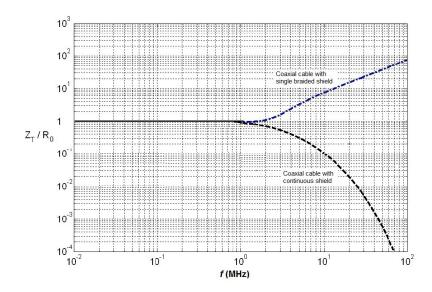
The graph in figure 62 shows how the impedance of a cable (with respect to DC-resistance  $R_0$ ) with mesh shield coincides with that of a continuous shield until the width of the openings becomes comparable to the wavelength of the disturbance, after which the two curves diverge and the mesh shield begins to lose its efficacy. The shield must be connected at both ends, otherwise it could act as a waveguide or antenna.
