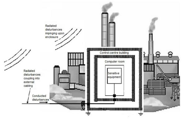
Figure 28: EMC for an industrial control center
