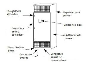
Figure 49: earthing with cable clamps
