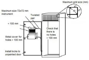
Figure 51: outline of EMC measures in a control panel
