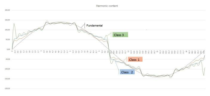
Figure 25: resulting waveform for the three classes
