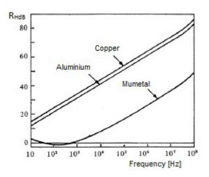
Figure 44: coefficient  $\mathrm{R}_{_{\mathrm{HdB}}}$  in relation to frequency for certain materials
