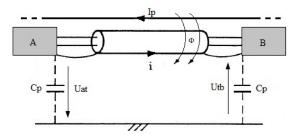
Figure 10: inductive coupling circuit
