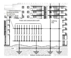
Figure 69: example of an earth connection in a building
