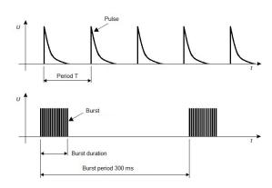
Figure 19: diagram of pulse burst
