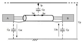
Figure 11: capacitive coupling circuit
