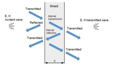
Figure 43: transmission of electromagnetic disturbances in a shield
