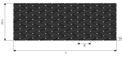
Figure 61: mesh shield
