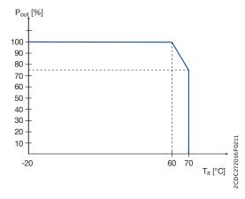
Characteristic curve of temperature at rated load
