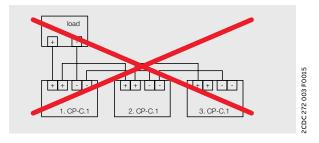
$Incorrect\ wiring\ for\ increased\ power$
