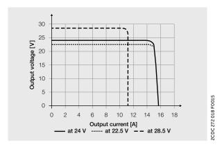
Characteristic curve of output at Ta = 25  $^{\circ}$ C
