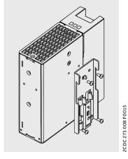
To mount the power supply in position 7 remove the DIN rail adapter that is fasten with 4 screws and attach it on the side of the power supply.
