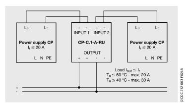
True redundancy using a CP-C.1-A-RU redundancy unit
