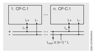
Simple redundancy or n+1 setup
