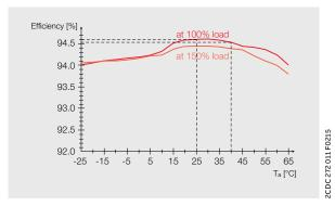
Typical efficiency over ambient temperature
