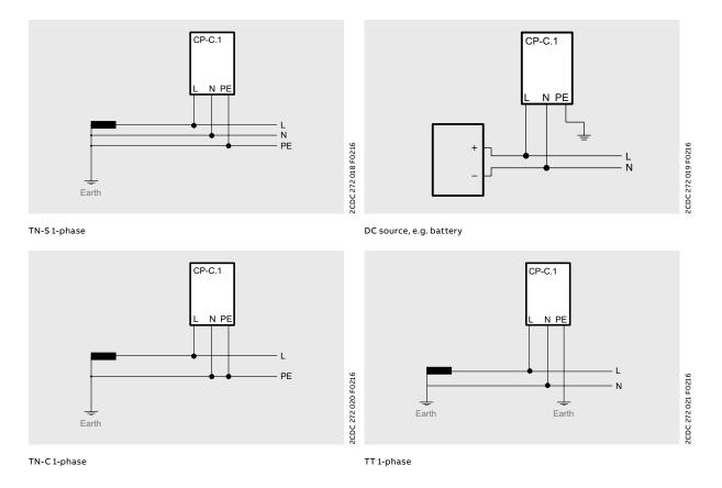
In AC networks the input voltage range is defined by -15...+10 % of the rated input voltage. However, in DC networks the rated input voltage is equal to the input voltage range.
