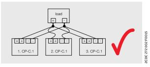
Correct wiring for increased power
