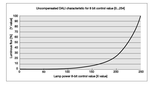
If a *DALI (logarithmic)* dimming curve is selected in the gateway, the KNX value relates to the 8-bit lamp power control value, the X value.
