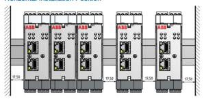
Ambient operating temperature (T<sub>A</sub>) and installation distance and position
