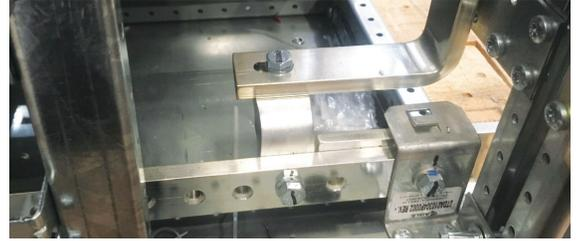
The ground bus bar is designed to use one single bar across the sections or the shipping pallet, this bus bar can be placed on the bottom of the units, or on the top of the units.
