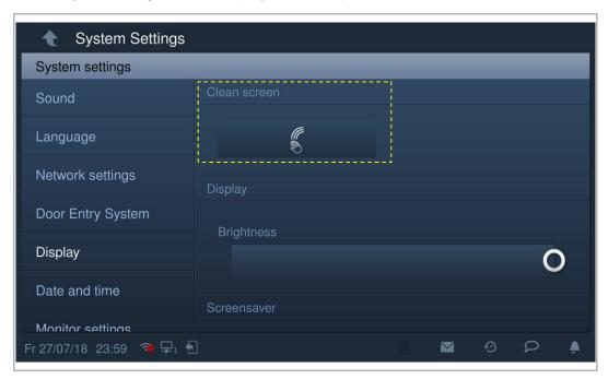
The countdown (1...30) is displayed on the screen. Any operations on the screen will be invalid. This device will exit "Clean screen" mode if an incoming call is received.
