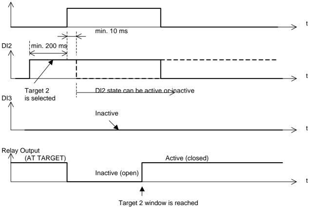
Figure 27. Positioning move from Target 1 to Target 2
