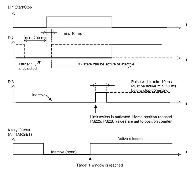
Figure 28. Positioning move from Target 2 to Target 1
