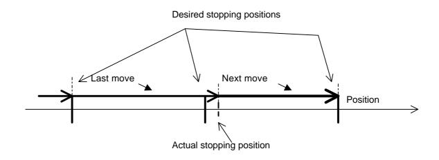
Figure 29. Application example 4, corrective action of position mode 4
