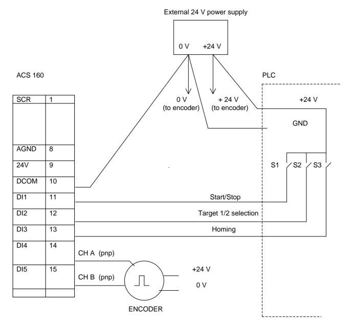
Figure 9. Encoder connection example 2
