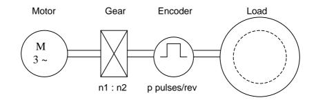
Figure 33. Encoder gear function when encoder is on the side of the load
