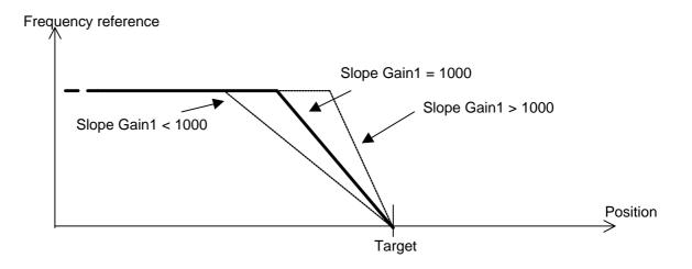
Figure 20. The effect of Slope gain 1 parameter
