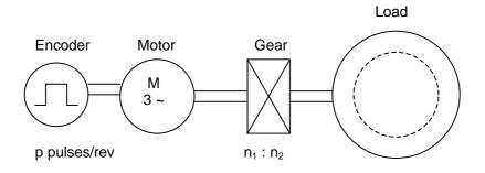
Figure 34. Encoder gear function when encoder is on the motor shaft
