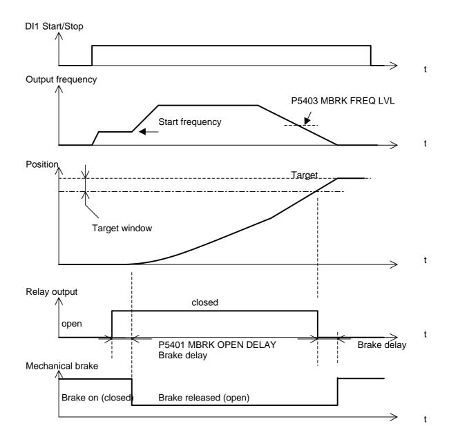
Figure 16. Operation of electromechanical brake control with positioning.
