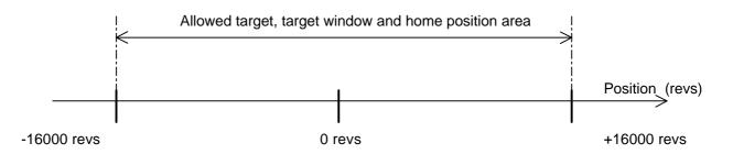
Figure 17. Target, target window and home position setting area
