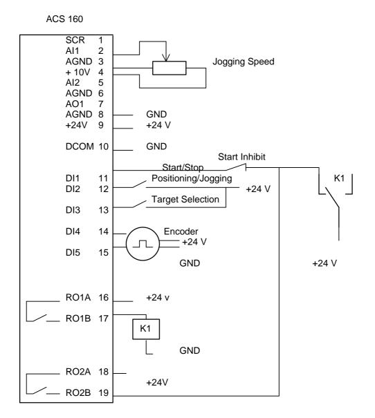
Figure 31. Application example 4, circuit diagram
