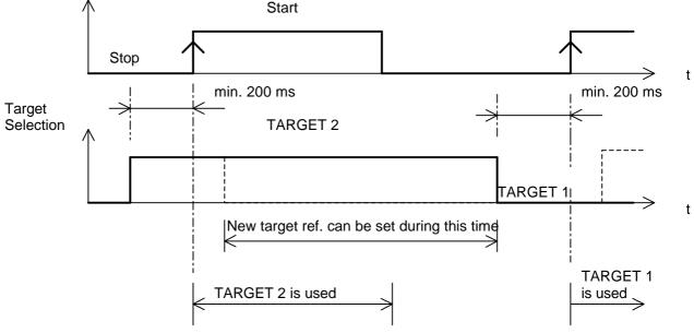
Figure 18. Timing of target reference selection.
