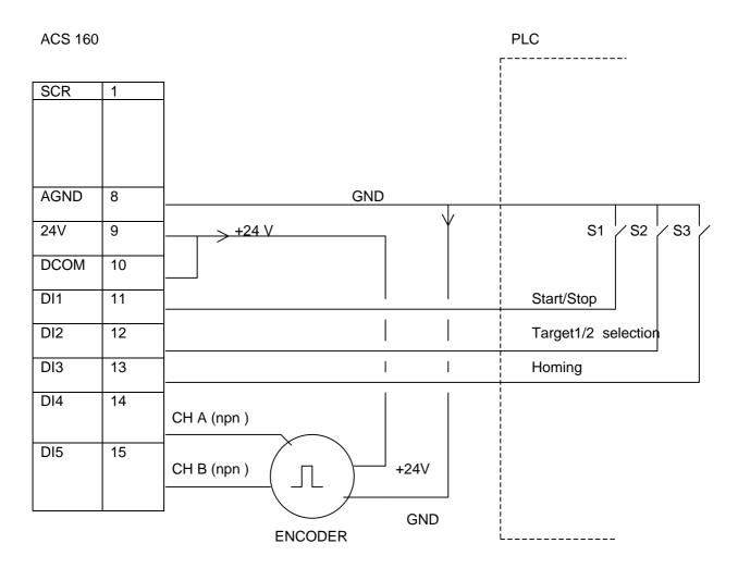
Figure 8. Encoder connection example 1
