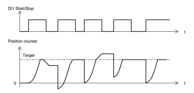
Figure 10. Relative move 1 mode with corrective action.
