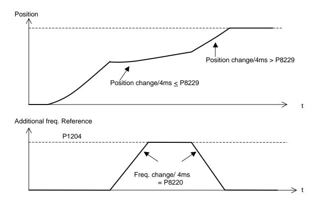
Figure 21. The effect of parameters 8220 and 8229.
