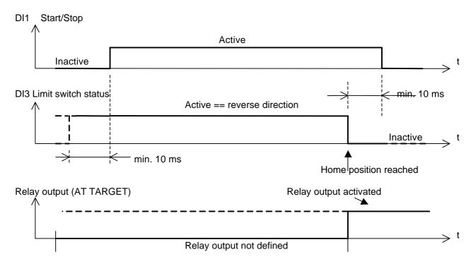
Figure 26. Homing timing diagram
