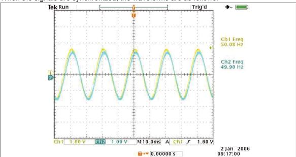
When there is a phase difference, the waveforms are as follows:
