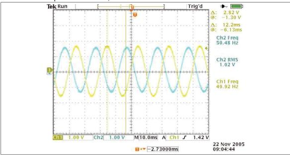
When the waveforms match, the unit gives a SYNC signal.
