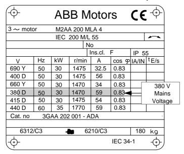
**Note:** Set the motor data exactly the same as on the motor nameplate. For example, if the motor nominal speed is 1440 rpm on the nameplate, setting the value of Parameter 99.08 MOTOR NOM SPEED to 1500 rpm results in wrong operation of the drive.
