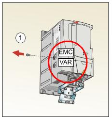
Note: In frame size R4 the EMC screw is located to the right of terminal W2.
