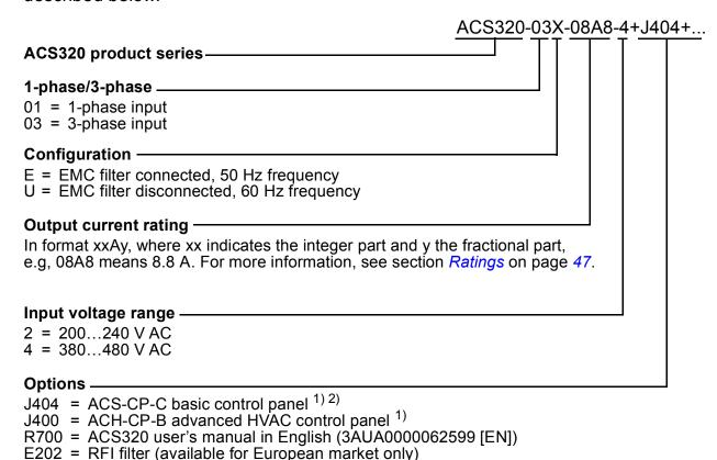
1) The ACS320 is compatible with panels that have the following panel revisions and panel firmware versions. To find out the revision and firmware version of your panel, see chapter Control panels, section Applicability in ACS320 user's manual (3AUA0000062599 [English]).
