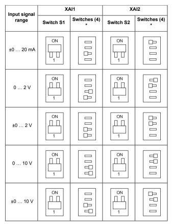
\* The voltage range switches are not in use when the corresponding input is operating in the current mode.
