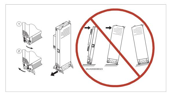
• To prevent the drive module from falling, attach its top lifting lugs with chains to the cabinet (1) before you push the module into the cabinet and pull it from the cabinet. Push the module into the cabinet and pull it from the cabinet carefully preferably with help from another person. Keep a constant pressure with one foot on the base of the module (2) to prevent the module from falling on its back.
