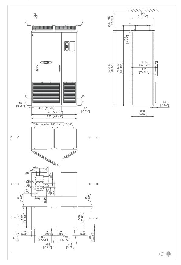
R11 IP22 (UL Type 1) and IP42 (UL Type 1 Filtered, option +B054)
