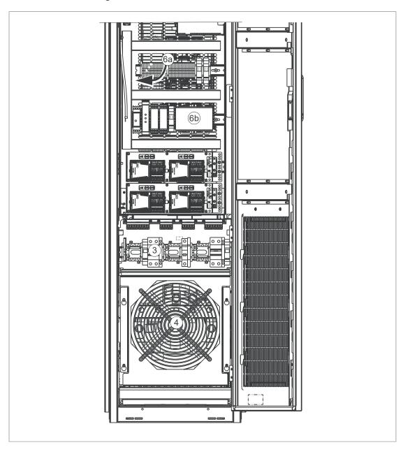
7. Route the cables to the control unit (a) and additional terminal block X504 (option +L504) and to options +QXXX, +MXXX, +L505 and +L506 as shown below.
