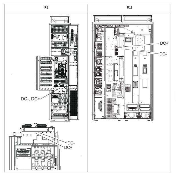
Make sure that the voltage between the drive DC busbars (+ and -) and the grounding (PE) busbar is close to 0 V.
