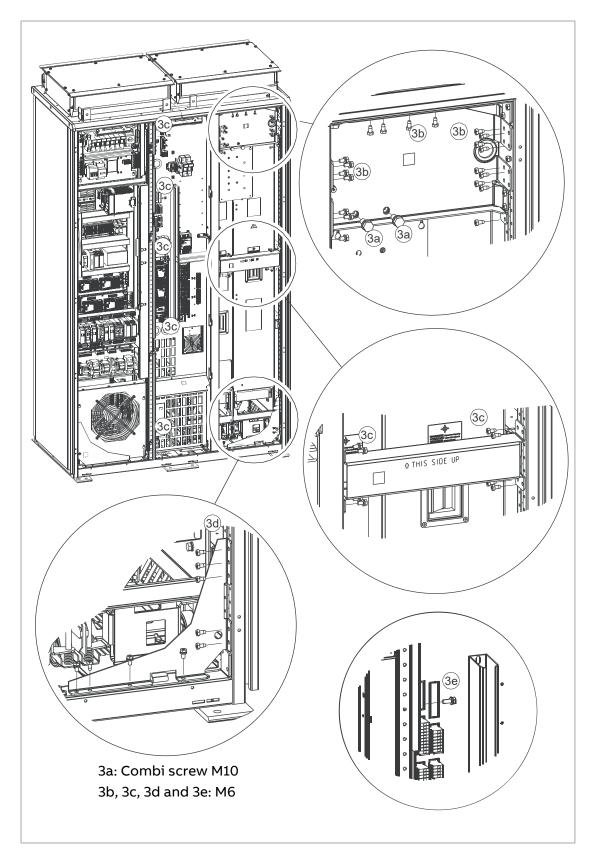
4. To open the module section swing-out frame, undo the M10 bolts from top and bottom (4 pcs).
