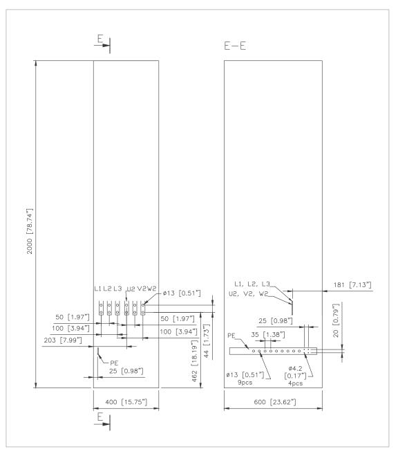
R8 input and motor cable terminal dimensions – bottom entry and exit
