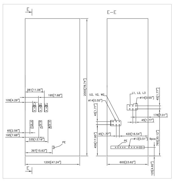
R11 input and motor cable terminal dimensions – bottom entry and exit
