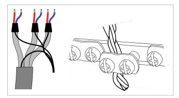
**Note:** At the other end of the cable, leave the shields unconnected or ground them indirectly via a high-frequency capacitor with a few nanofarads, eg. 3.3 nF / 630 V. The shield can also be grounded directly at both ends if they are in the same ground line with no significant voltage drop between the end points.
