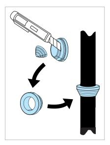
8. Attach the conductive sleeves to the cable shields with cable ties.
