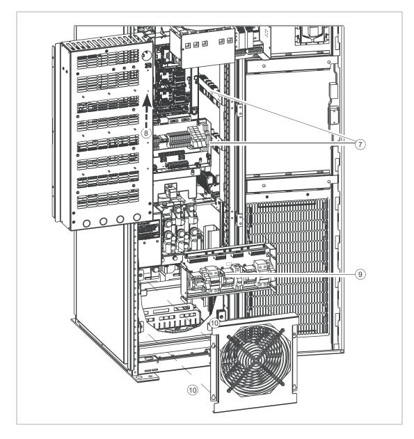
11. Loosen the four M5 screws and remove the plastic shroud.
