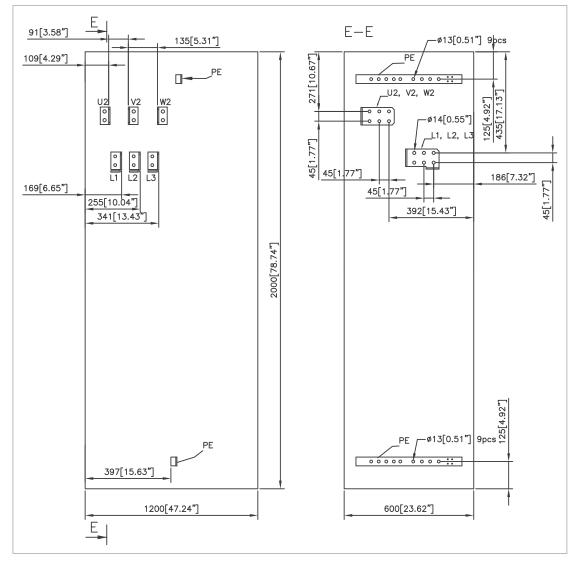
R11 input and motor cable terminal dimensions – top entry and exit (options +H351 and +H353)
