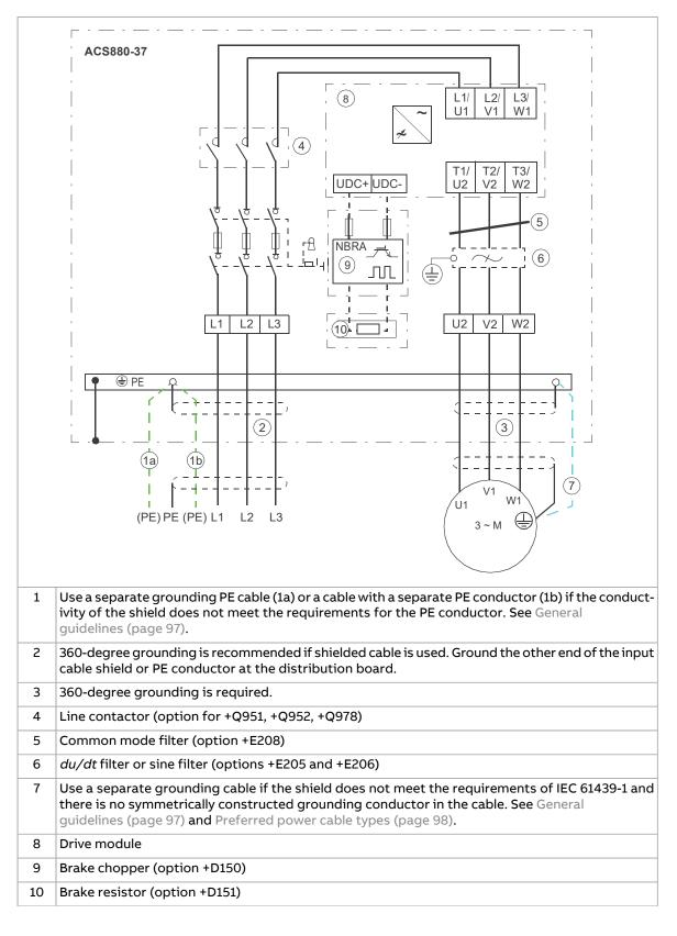
**Note:** If there is a symmetrically constructed grounding conductor on the motor cable in addition to the conductive shield, connect the grounding conductor to the grounding terminal at the drive and motor ends. Do not use an asymmetrically constructed motor cable. Connecting its fourth conductor at the motor end increases bearing currents and causes extra wear.
