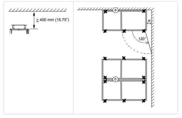
**Note 1:** Any height adjustment must be done before attaching the cabinet sections to the floor or to each other. Height adjustment can be done by using metal shims between the cabinet bottom and floor.
