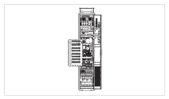
3. Undo the memory unit mounting screw and take the memory unit out. Replace the unit in reverse order. Note: There is a spare screw next to the memory unit slot.
