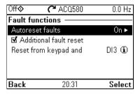
The Fault functions submenu contains settings for resetting faults automatically or manually.
