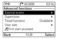
The Advanced functions submenu contains settings for advanced functions, such as triggering or resetting custom faults via I/O, signal supervision, using the drive with timed functions, or switching between several entire sets of settings. In addition you can run the First start assistant from this submenu.
