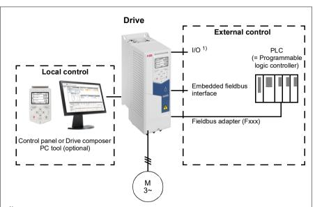
1) Extra inputs/outputs can be added by installing an optional I/O extension module (CMOD-01, CMOD-02, CHDI-01, CPTC-02, or CAIO-01) in drive slot.
