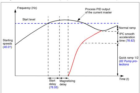
The timing diagram of smooth pump transitions shows the pump starting steps. In this case, the process PID output of the current master has exceeded the start level (76.30...76.36).
