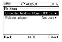
Use the Fieldbus menu to set up and view communication through embedded fieldbus or fieldbus adapter.
