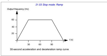
If the acceleration time is too short, the drive may trip out on overcurrent. If the deceleration ramp is set to stop too quickly, the drive may trip out on overvoltage. These scenarios are unlikely in most applications due to the internal current and voltage limiting features built into the drive. However, the desired ramps times will not be achieved in such circumstances.
