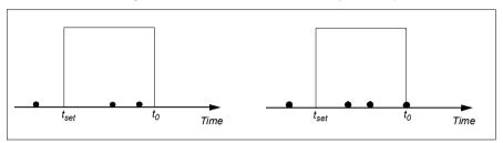
The third pump cleaning cycle starts within the preset count time (one hour) and the pump cleaning function trips on a fault and the pump is stopped without performing the third cleaning cycle. After reseting fault, the drive starts with the third pump cleaning cycle.
