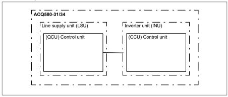
The supply unit can be controlled through the inverter unit. For example, the inverter unit can send a control word and references to the supply unit, enabling the control of both units from the interfaces of one control program.
