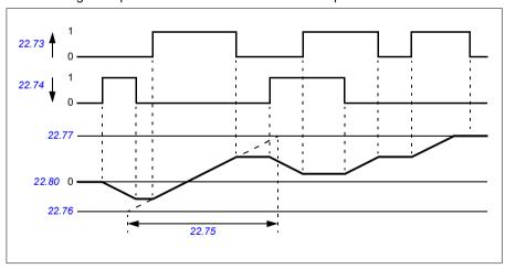
Parameters 22.73 Motor potentiometer up source and 22.74 Motor potentiometer down source control speed or frequency from zero to maximum speed or frequency.
