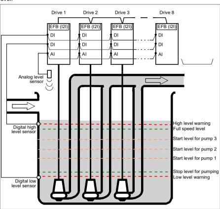
The first pump (master) will start when the actual level is above the start point 1. More pumps will start and stop based on the rising (emptying) or falling (filling) water levels of individual pumps. In case of a pump failure or if drive is disconnected for maintenance, the system continues operation with the remaining pumps and drives.
