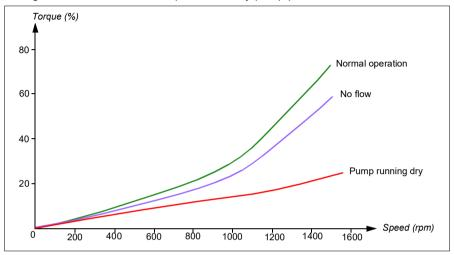
The dry pump can be detected using the underload curve, low level mechanical switch and pressure sensor.
