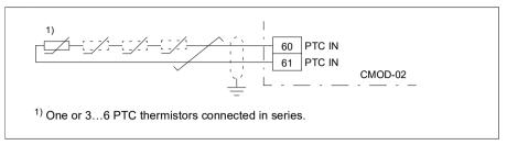
The resistance of the PTC sensor increases when its temperature rises. The increasing resistance of the sensor decreases the voltage at the input, and eventually its state switches from 1 to 0, indicating overtemperature.
