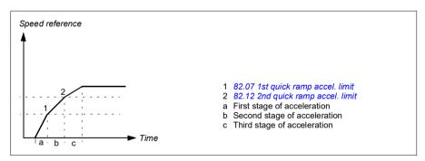
In submersible (a.k.a borehole) pumps, the mechanical wearing of bearings can be reduced by ramping the pump quickly to a certain speed.
