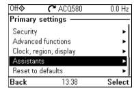
The Assistants submenu includes a variety of assistants that can be used to configure the drive.
