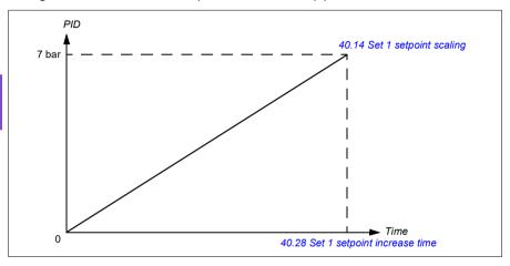
If the pumping system is leaking or is damaged then the setpoint will not reach in time. To detect such a condition, you can enable soft pipe fill supervision to generate a warning or a fault. The time is calculated with the last reference change in parameter 40.03 Process PID setpoint actual.
