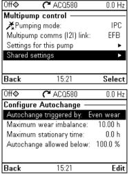
Multipump (IPC, intelligent pump control) systems allows up to 8 drives to be connected to each other. This menu contains programming assistants for load sharing, balancing the run time between the pumps and keeping each pump running optimally.
