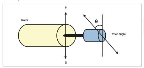
The autophasing routine is performed with permanent magnet synchronous motors to determine the rotor angle at every start.
