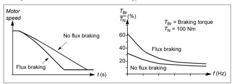
The drive monitors the motor status continuously, also during flux braking. Therefore, flux braking can be used both for stopping the motor and for changing the speed. The other benefits of flux braking are:
